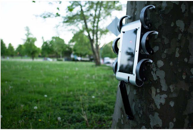
Fig. 8. The T-RHex platform statically hanging from a Sycamore tree.
