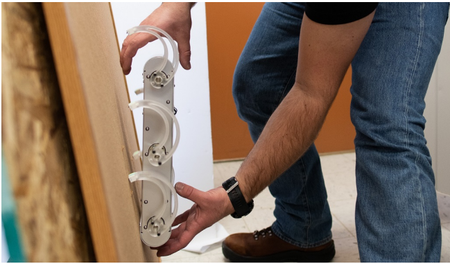
Fig. 6. A static slope cling test in which the robot is hanging entirely by the back legs after initial tip. The cork test surface is shown here.
