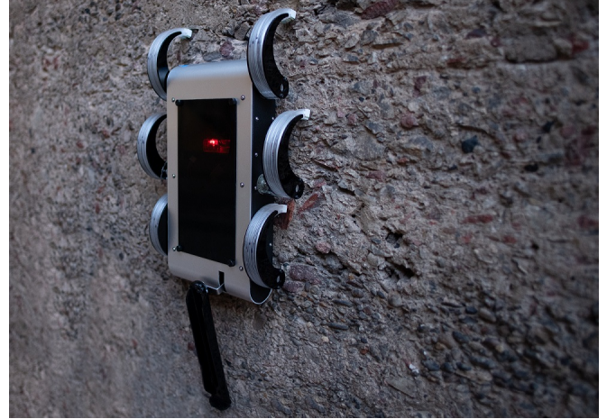
Fig. 1. The new T-RHex robot platform statically clinging to rough aggregate concrete. Each leg includes 9 individually compliant microspines.
