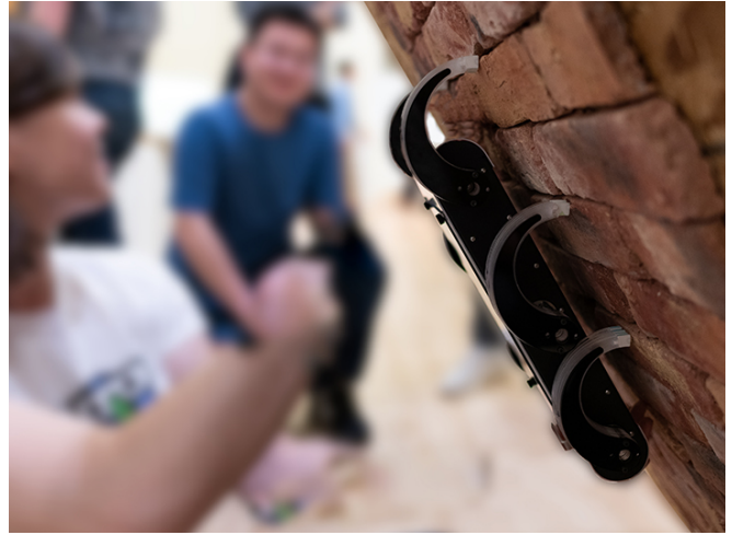
Fig. 5. T-RHex hanging from brick facade with a steep overhang. The maximum static cling angle recorded during experiments was 116^\circ and reached a further 135^\circ when placed by hand.
