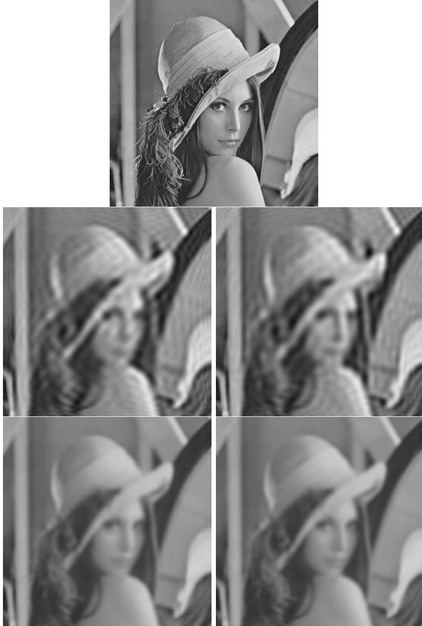
FIG. 2. Top: original image. Middle: least squares in (55) basis (left) and (59) basis (right). Bottom: Radon–Nikodym in (55) basis (left) and (59) basis (right). The bases (55) and (59) are of 2500 elements ( n_x = n_y = 50 ) and 2485 elements ( n = 3 , \mathcal{D} = 69 ) respectively.
