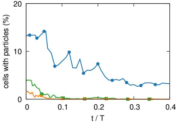
Figure 25: Percentage of interfacial cells where the curvature is computed with particles for  $R/h = 9.6$  (blue circles), 19.2 (green squares), 38.4 (orange triangles).
