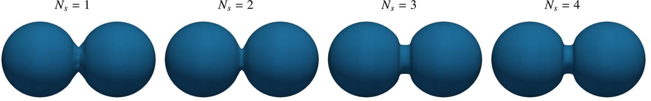
Figure 7: Isosurfaces of the volume fraction with  $R/h = 19.2$  at  $t/T = 0.08$  depending on the number of cross sections  $N_s = 1, 2, 3$  and  $4$ .
