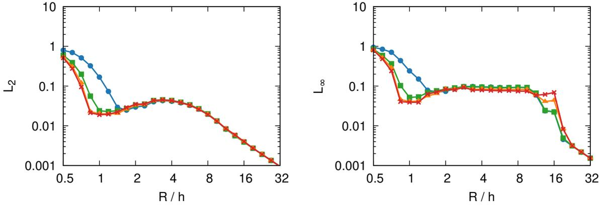
Figure 4: Curvature error for a sphere in  $L_2$  and  $L_\infty$  norms depending on the resolution for various values of the number of particles  $N = 3$  (blue circles),  $5$  (green squares),  $7$  (orange triangles) and  $9$  (red crosses).
