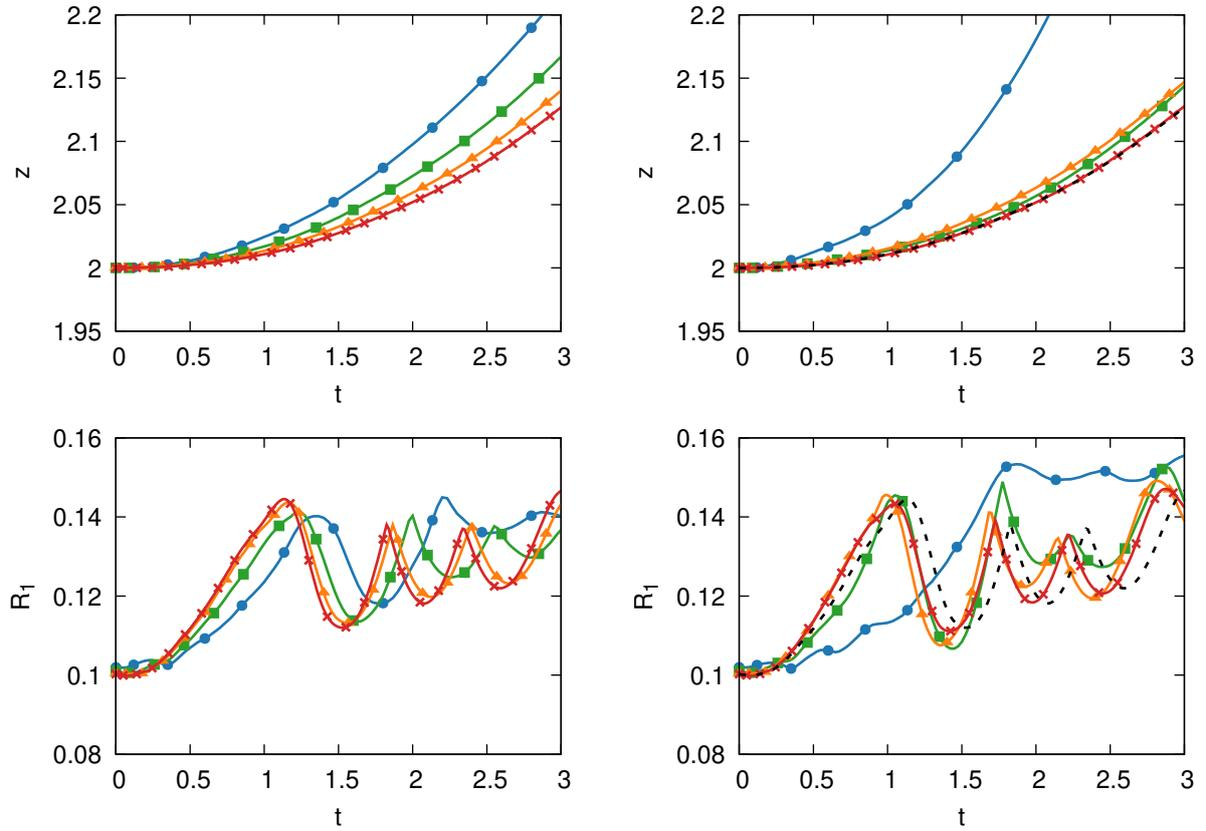
Figure 19: Trajectory of the droplet center of mass in the  $z$ -direction and the smallest semi-axis of the ellipsoid of gyration at various resolutions  $R/h = 1.53$  (—●—), 2.04 (—■—), 3.06 (—▲—) and 4.08 (—×—): present (left) and GHF (right). The dashed line - - - on the right shows the results at the finest resolution  $R/h = 4.08$  by the present method.
