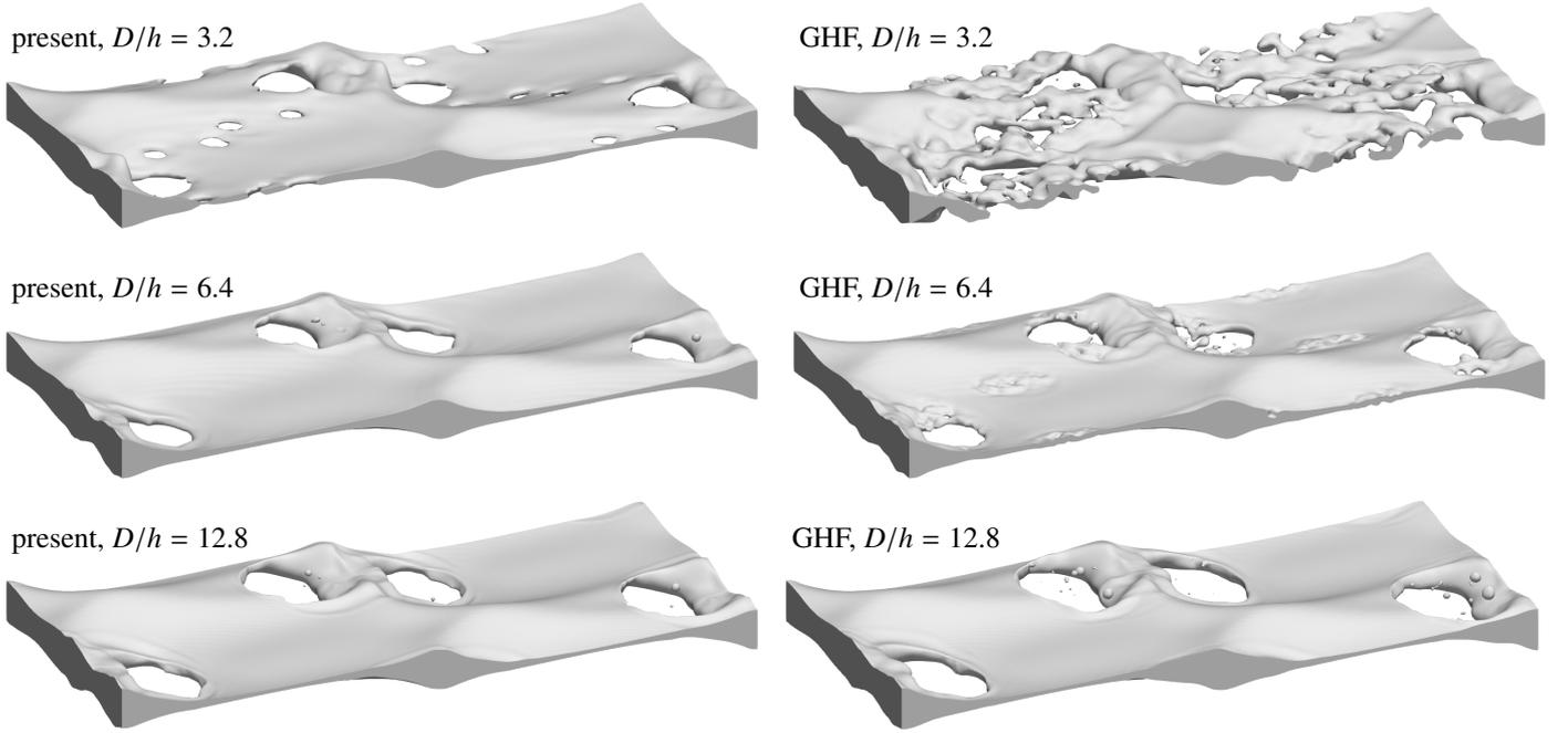
Figure 27: Shapes of the air sheet at  $t = 1.7$  computed with present method (left) and GHF (right) at resolutions  $D/h = 3.2$  (top), 6.4 (middle) and 12.8 (bottom).
