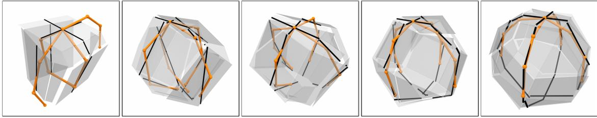
Figure 9: Polygons of the interface, cross sections (black) in case  $N_s = 2$  and positions of particles (orange) from one selected cell for a sphere at resolutions  $R/h = 0.59, 0.71, 0.84, 1.0$  and  $1.19$ .
