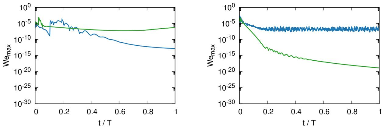
Figure 13: Evolution of the velocity error for a static droplet in 3D at resolutions  $R/h = 2$  (left) and 4 (right): present  $\text{---}$  and GHF  $\text{---}$ .
