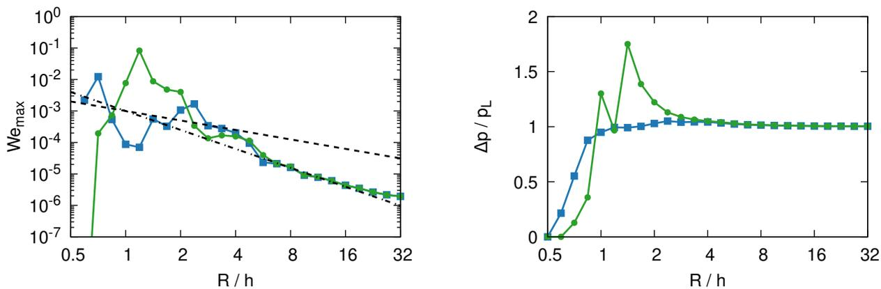
Figure 14: Velocity error and the pressure jump for a translating droplet in 2D depending on the resolution: present  $\blacksquare$  and GHF  $\bullet$ . Convergence with first  $---$  and second  $- \cdot -$  order.
