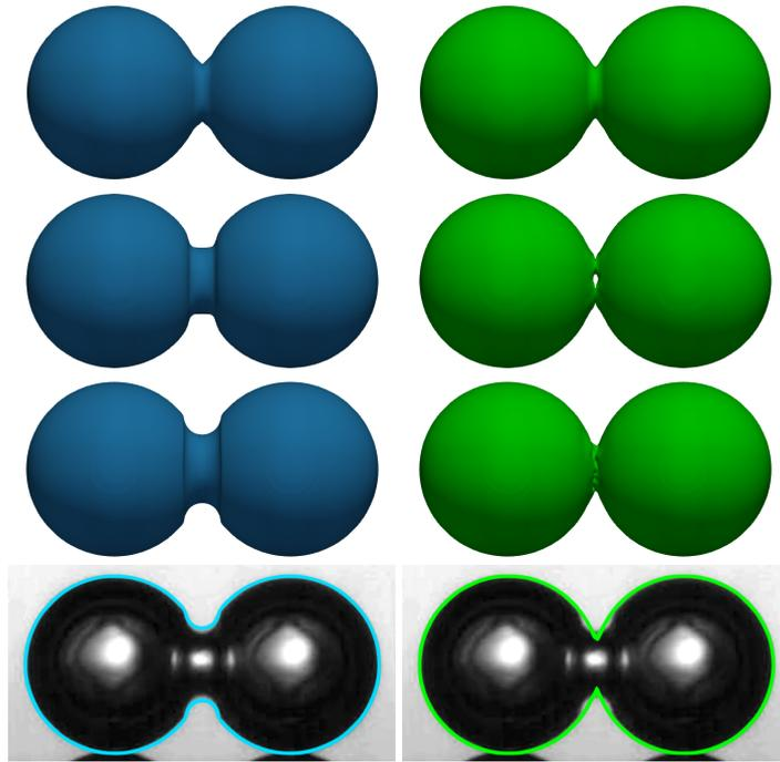
Figure 22: Isosurfaces of volume fraction at  $t/T = 0.08$  depending on resolution  $R/h = 9.6$  (top),  $19.2$  (middle) and  $38.4$  (bottom): present (left) and GHF (right). Experimental image [35] overlapped with contours from the finest mesh of each method. The time value for the experimental image is multiplied by  $1.2$ .
