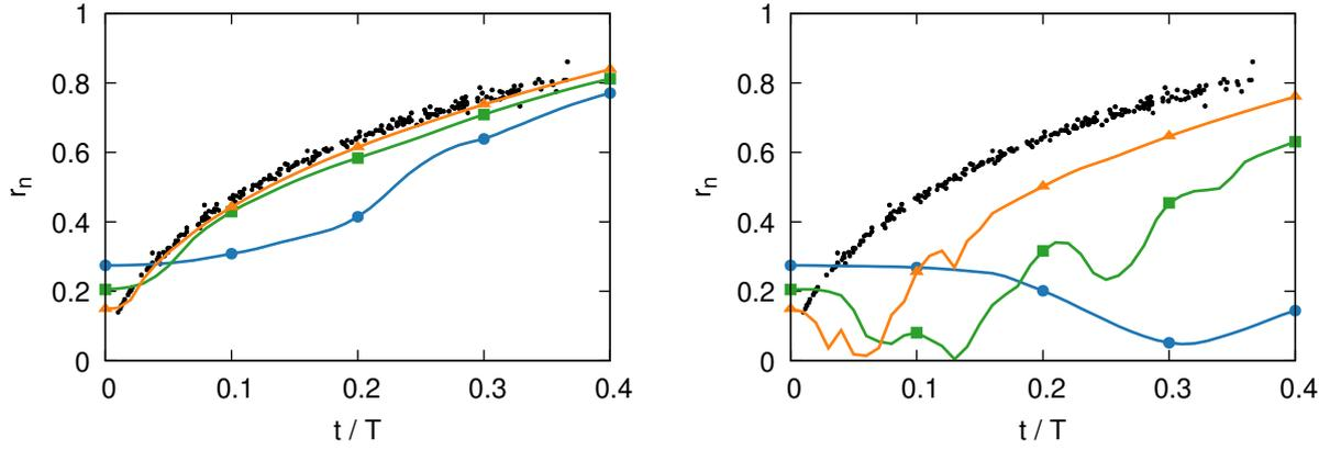
Figure 24: Evolution of the neck radius depending on the resolution  $R/h = 9.6$  (blue circles), 19.2 (green squares), 38.4 (orange triangles): present (left) and GHF (right) compared to experiment [35] (dots).
