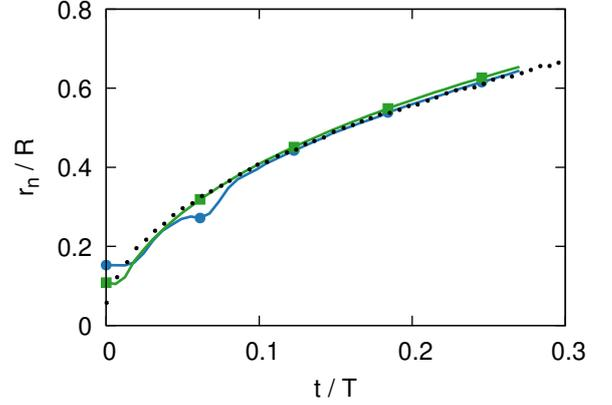
Figure 33: Evolution of the coalescence neck radius relative to the bubble radius depending on the resolution  $R/h = 38.4$  (—) and  $76.8$  (—) produced by Aphros compared to experiment [39] (dots).
