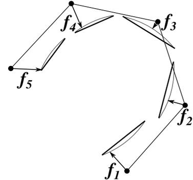
Figure 28: Line segments represent the interface and circular arcs of curvature  $\kappa$  pass through their endpoints. The force acts on each particle towards the circular arc from the nearest line segment.
