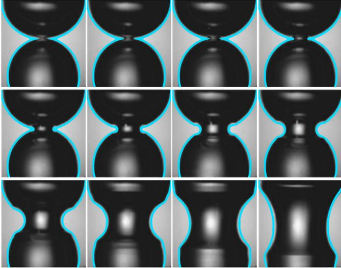
Figure 32: Snapshots from experiment [39] overlaid by the projections of the shapes from the simulation by Aphros with resolution  $R/h = 76.8$  (blue lines) at times  $t/T = 0, 0.0061, 0.012, 0.018, 0.031, 0.043, 0.061, 0.08, 0.12, 0.17, 0.21$  and  $0.27$ . Experimental images reprinted from [39], with the permission from AIP Publishing.
