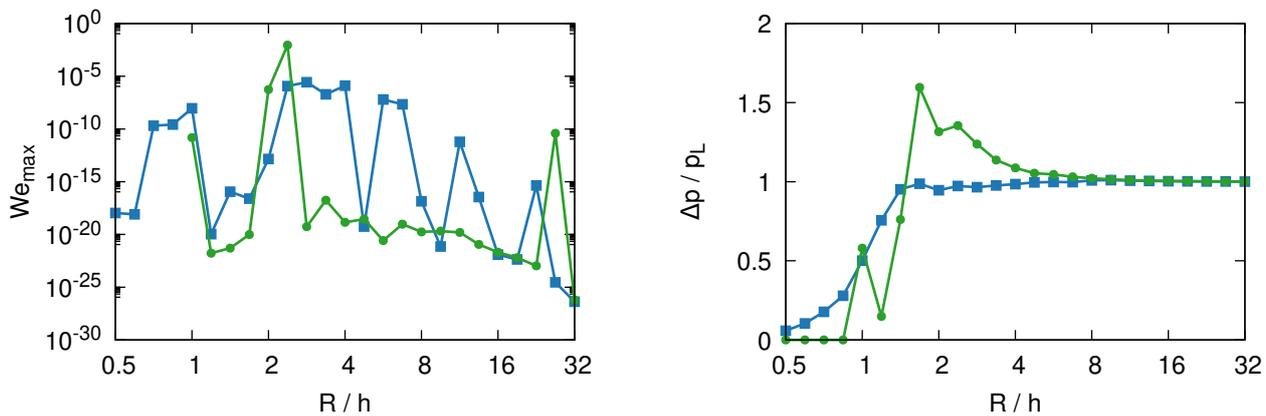
Figure 12: Velocity error and the pressure jump for a static droplet in 3D depending on the resolution: present  $\blacksquare$  and GHF  $\bullet$ .
