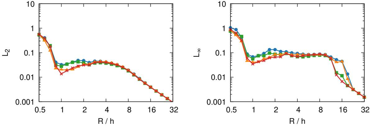
Figure 5: Curvature error for a sphere in  $L_2$  and  $L_\infty$  norms depending on the resolution for various values of the number of cross sections  $N_s = 1$  (blue circles),  $2$  (green squares),  $3$  (orange triangles) and  $4$  (red crosses).
