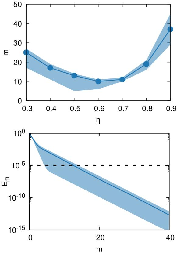
Figure 3: Equilibration of particles on a sphere at resolution  $R/h = 4$ . The number of iterations required to reach the convergence criterion (10) with  $\varepsilon_p = 10^{-5}$  depending on the relaxation factor  $\eta$  (top) and the convergence history for the difference after one iteration with  $\eta = 0.5$  (bottom). The lines show the median and the shades show the 10% and 90% percentiles over the interfacial cells.
