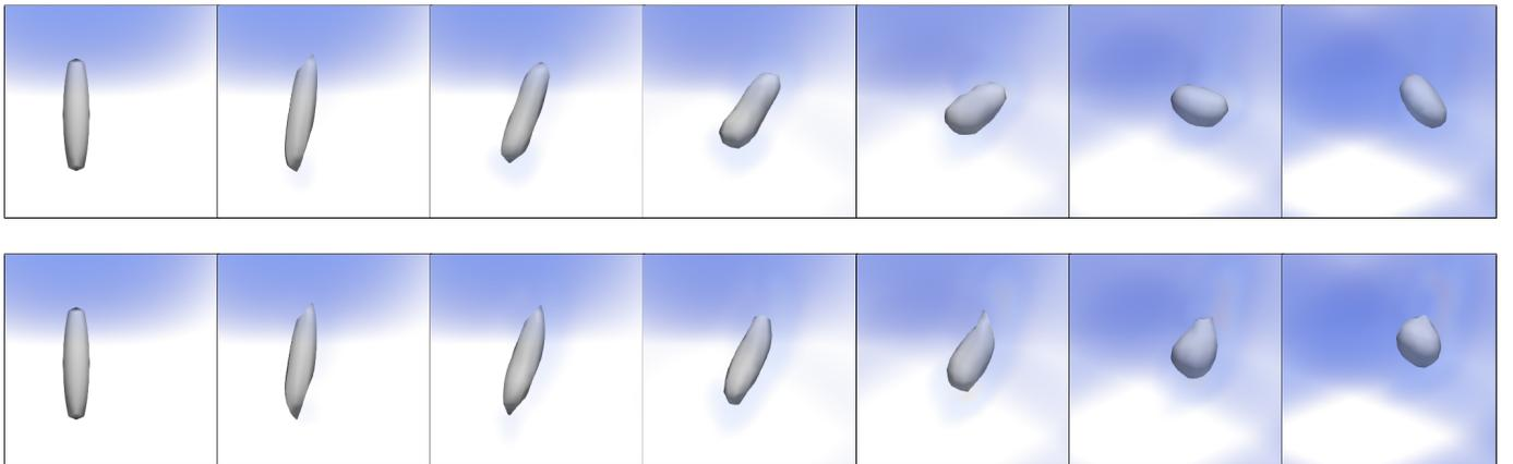
Figure 20: Isosurfaces of the volume fraction and the magnitude of vorticity (increasing values from blue to red) with resolution  $R/h = 1.53$  at  $t = 0.0, 0.3, 0.6, 0.9, 1.2, 1.5$  and  $1.8$ : present method (top) and GHF (bottom). Unlike GHF, our method captures the oblate shape at  $t = 1.5$ .
