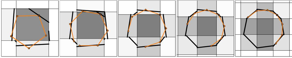
Figure 8: Line segments of the interface (black) and positions of particles (orange) from one selected cell for a circle at resolutions  $R/h = 0.59, 0.71, 0.84, 1.0$  and  $1.19$ . The central particle is highlighted by a thicker edge.
