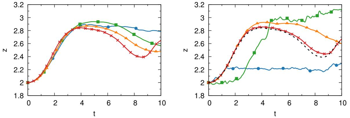
Figure 17: Trajectory of the bubble center of mass in the  $z$ -direction at various resolutions  $R/h = 1.53$  —●—,  $2.04$  —■—,  $3.06$  —▲— and  $4.08$  —×—: present (left) and GHF (right). The dashed line - - - on the right shows the trajectory at  $R/h = 4.08$  from the present method.
