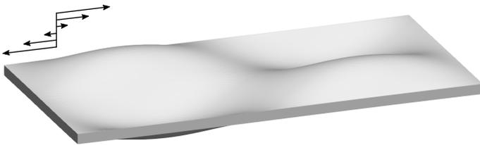
Figure 26: Initial volume fraction representing an air sheet. Arrows indicate the direction of the shear.
