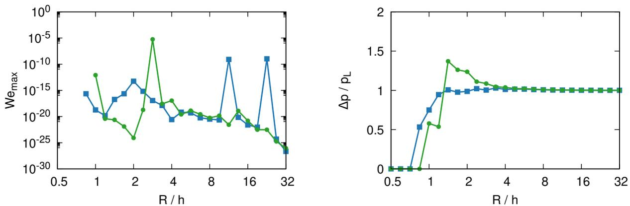
Figure 11: Velocity error and the pressure jump for a static droplet in 2D depending on the resolution: present  $\blacksquare$  and GHF  $\bullet$ .
