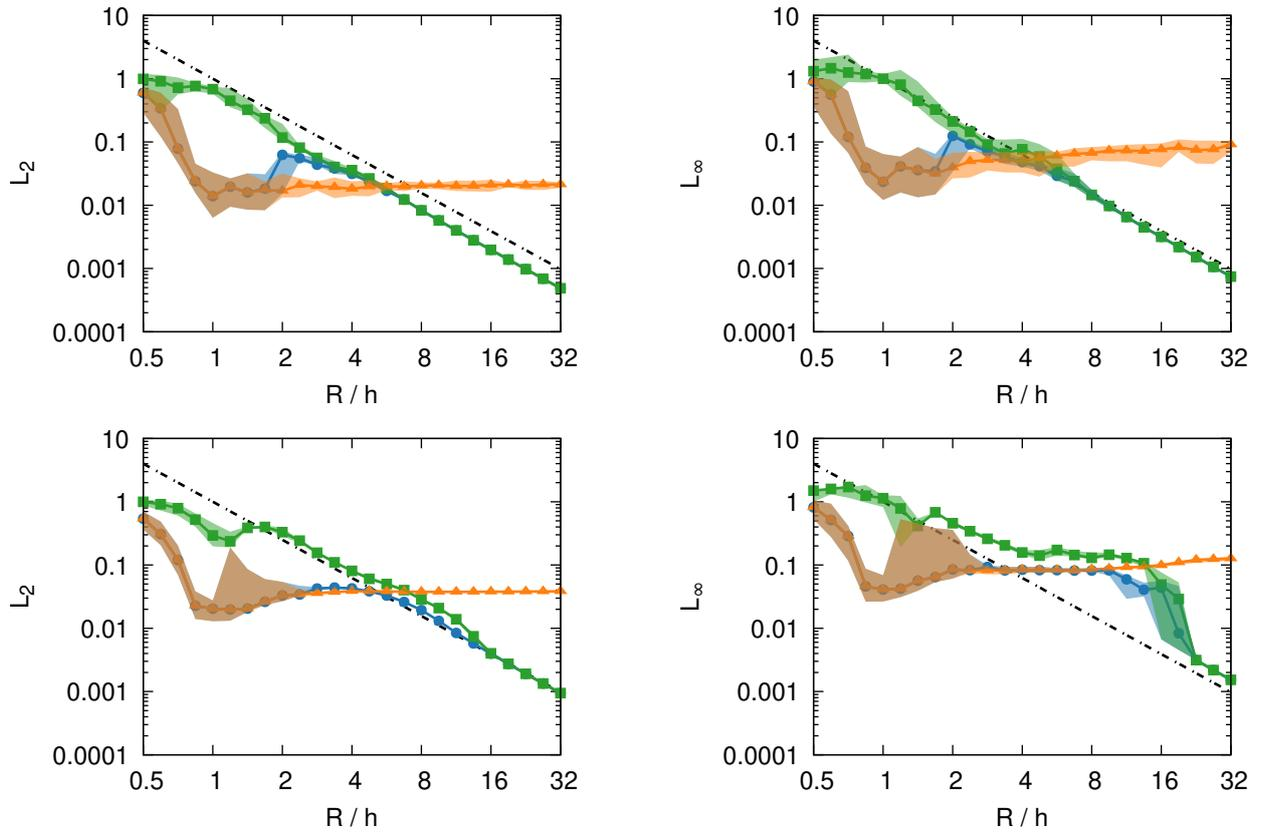
Figure 10: Curvature error for a circle (top) and sphere (bottom) in  $L_2$  and  $L_\infty$  norms depending on the resolution: particles only  $\text{---}\blacktriangle\text{---}$ , combined particles and heights  $\text{---}\bullet\text{---}$ , GHF  $\text{---}\blacksquare\text{---}$  and second-order convergence  $\text{---}\text{---}\text{---}$ . The lines show the median and the shades show the 10% and 90% percentiles for random positions of the center.
