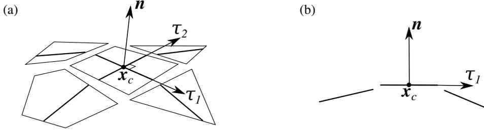
Figure 2: Curvature estimation in three dimensions in case  $N_s = 2$ . (a) Interface polygons with the cross sections. (b) One cross section in local two-dimensional coordinates.
