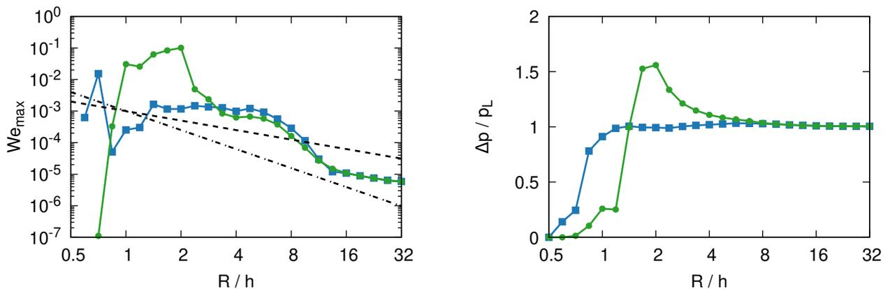
Figure 15: Velocity error and the pressure jump for a translating droplet in 3D depending on the resolution: present  $\blacksquare$  and GHF  $\bullet$ . Convergence with first  $---$  and second  $- \cdot -$  order.
