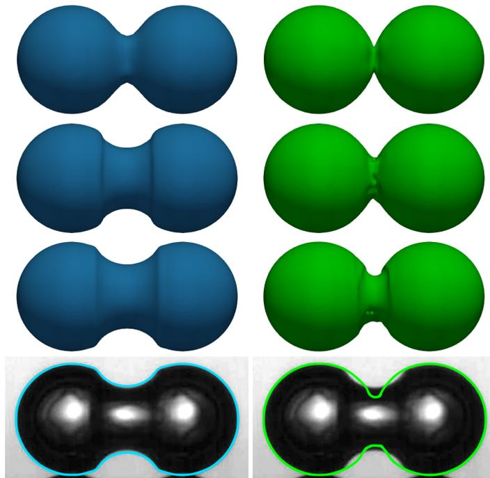
Figure 23: Isosurfaces of volume fraction at  $t/T = 0.18$  depending on resolution  $R/h = 9.6$  (top),  $19.2$  (middle) and  $38.4$  (bottom): present (left) and GHF (right). Experimental image [35] overlapped with contours from the finest mesh of each method. The time value for the experimental image is multiplied by  $1.2$ .
