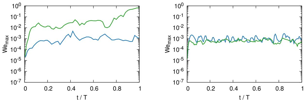
Figure 16: Evolution of the velocity error for a translating droplet in 3D at resolutions  $R/h = 2$  (left) and  $4$  (right): present  $---$  and GHF  $---$ .
