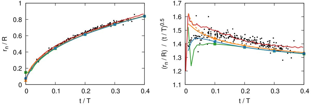
Figure 31: Evolution of the coalescence neck radius relative to the bubble radius (left) and the coalescence neck radius divided by  $\sqrt{t}$  (right). Gerris in the axisymmetric formulation with adaptive mesh refinement with the equivalent resolution  $R/h = 307.2$  (---) and  $R/h = 614.4$  (—), Basilisk with proposed method for curvature at  $R/h = 38.4$  (—) and Aphros at  $R/h = 153.6$  (—). Experiment [35] (dots) and boundary integral [35] (—) without scaling of time.
