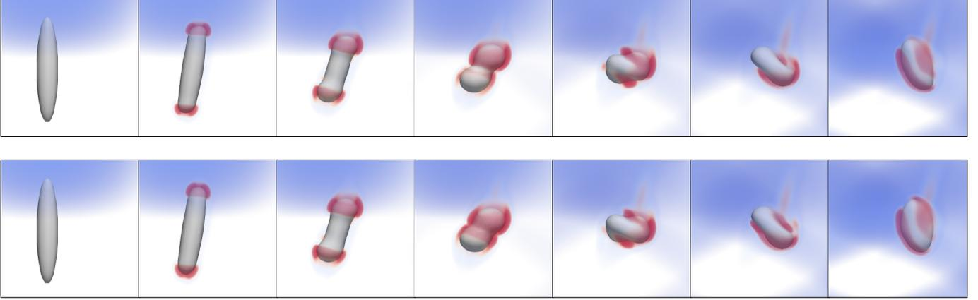
Figure 21: Isosurfaces of the volume fraction and the magnitude of vorticity (increasing values from blue to red) with resolution  $R/h = 4.08$  at  $t = 0.0, 0.3, 0.6, 0.9, 1.2, 1.5$  and  $1.8$ : present method (top) and GHF (bottom).
