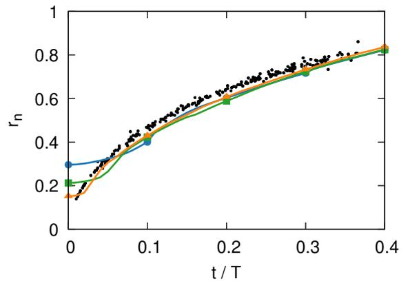
Figure 30: Evolution of the coalescence neck radius relative to the bubble radius depending on the resolution  $R/h = 9.6$  (blue circles),  $19.2$  (green squares) and  $38.4$  (orange triangles) produced by Aphros compared to experiment [35] (dots).
