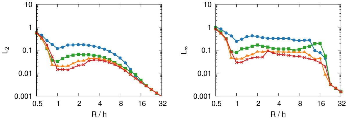
Figure 6: Curvature error for a sphere in  $L_2$  and  $L_\infty$  norms depending on the resolution for various values of the particle string length  $H_p = 2$  (blue circles),  $3$  (green squares),  $4$  (orange triangles) and  $5$  (red crosses).
