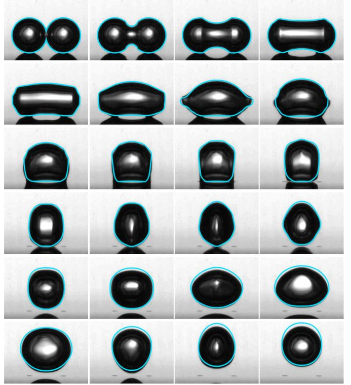
Figure 29: Snapshots from experiment [35] overlaid by the projections of the shapes from the simulation by Aphros with resolution  $R/h = 76.8$  (blue lines) at times  $t/T = 0, 0.13, 0.26, 0.4, 0.53, 0.66, 0.79, 0.92, 1.1, 1.2, 1.3, 1.4, 1.6, 1.7, 1.8, 2.1, 2.4, 2.6, 2.9, 3.2, 3.7, 4.2, 4.7$  and  $5.3$ . The time values for the experimental images are multiplied by 1.2.
