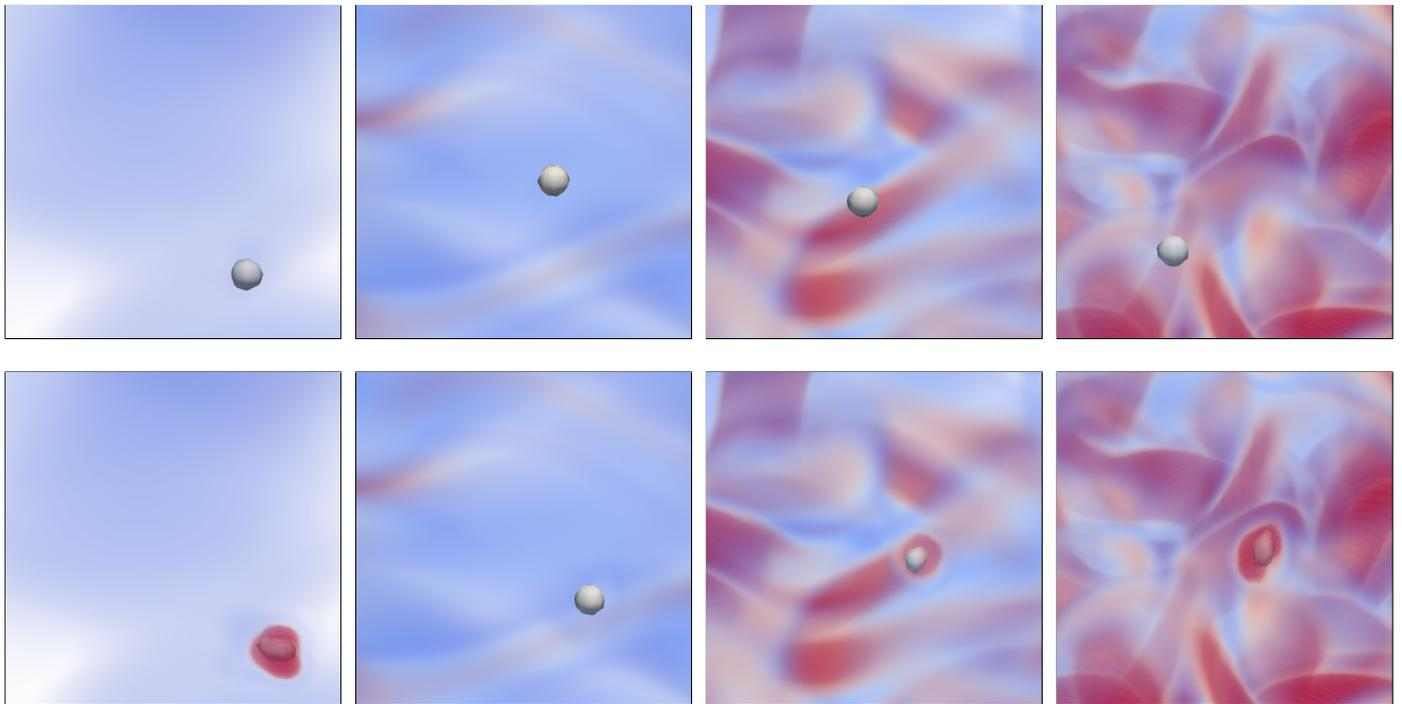
Figure 18: Isosurfaces of the volume fraction and the magnitude of vorticity (increasing values from blue to red) with  $R/h = 2.04$  at  $t = 1.0, 3.5, 6.0$  and  $8.5$ . At such resolution GHF (bottom) produces a solution with stronger spurious flow near the bubble than our method (top).
