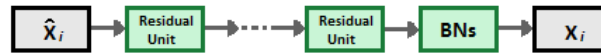
Fig. 3: The refiner network with the tensor size same throughout the network and deterministic binary neurons.
