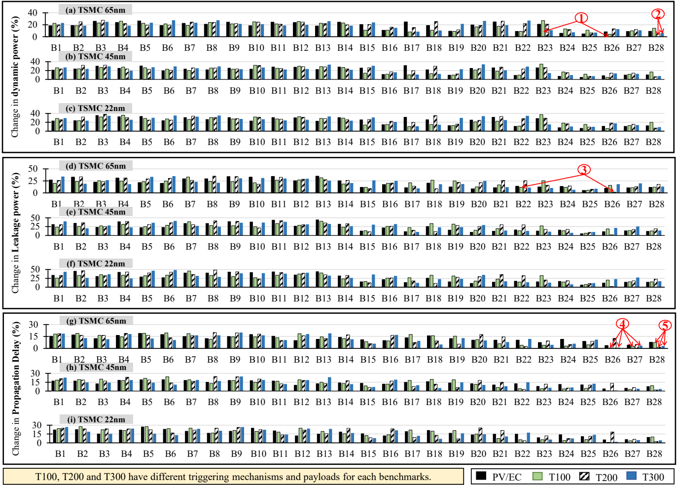
Fig. 9: Effects of process variations/Environmental Changes (PV/EC) on side-channel parameters, i.e., propagation delay, dynamic and Leakage power, on different ISCAS89 benchmarks in the presence of trust-hub benchmarks. Note, in these experiments, process variations are modeled by non-deterministically choosing the thickness oxide ( t_{ox} ), S/D junction depth, and threshold voltage from a given range. We use 65nm, 45nm, and 22nm TSMC CMOS models to extract the ranges of these parameters. It also shows that for designing a stealthy HT, it must be inserted deeper (to minimize the triggering probabilities) in the circuits and inserted in parallel (to minimize the effect on delay and dynamic power) to the computational path. In this analysis, we observed that different technologies have an impact on side-channel parametric behavior, but it does not affect the outcome of the security vulnerability analysis.
