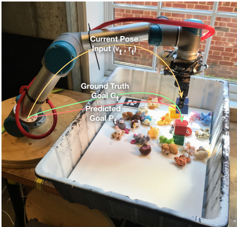
Fig. 2: The CoSTAR system [2] collecting the block stacking dataset. Each example consists of an attempt to stack 3 colored blocks in a specified order.
