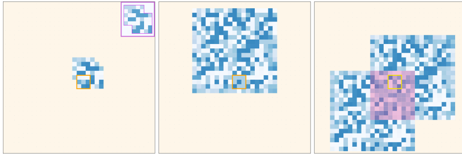
Fig. 6: Sensorimotor prediction with a static environment ( p_{env} = 0 ): Left: prediction of the pixels corresponding to a proto-object. Center: the entire environment learned by the agent. Right: given the input state, the prediction associated with some specific movements is ambiguous. The corresponding pixels are highlighted in red. For those, several predictions can contradict each other.
