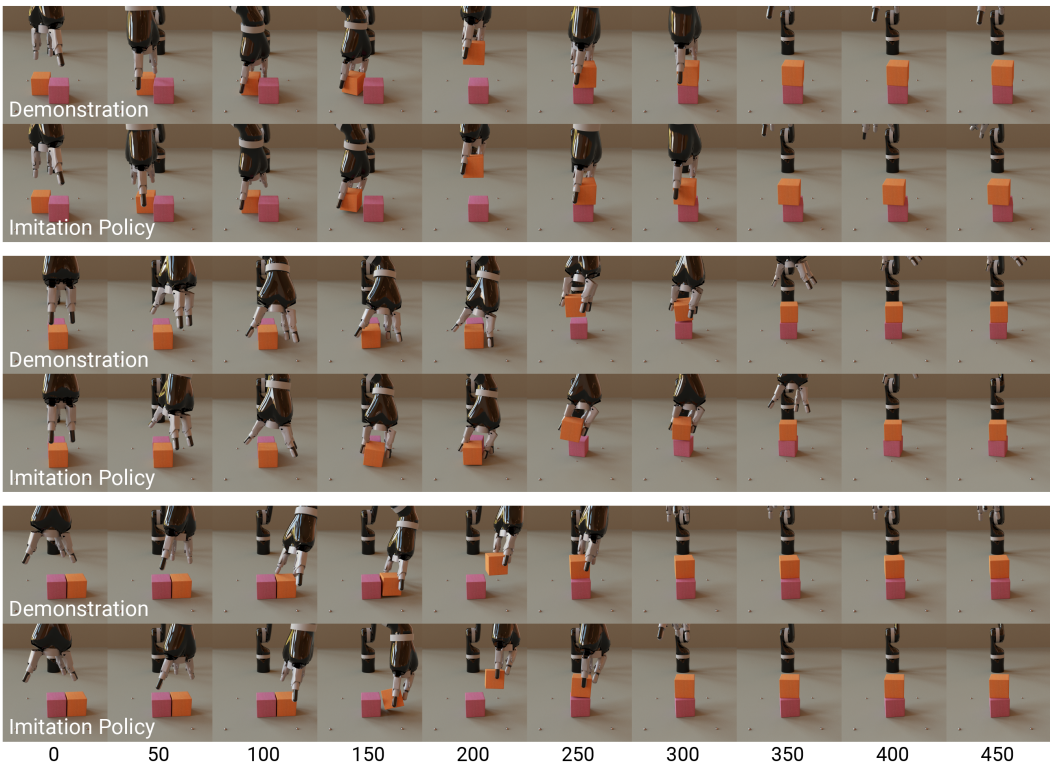
Figure 4: One-shot high-fidelity imitation. Given novel, diverse, test-set demonstration videos (three examples are shown above), the imitation policy is able to closely mimic the human demonstrator. In particular, it successfully maps image observations to arm velocities while managing the complex interaction forces among the arm, blocks and ground.
