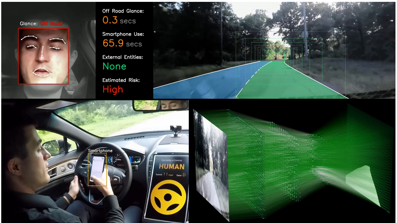
(a) Example of elevated risk under manual control during a period of frequent off-road glances to the smartphone.
