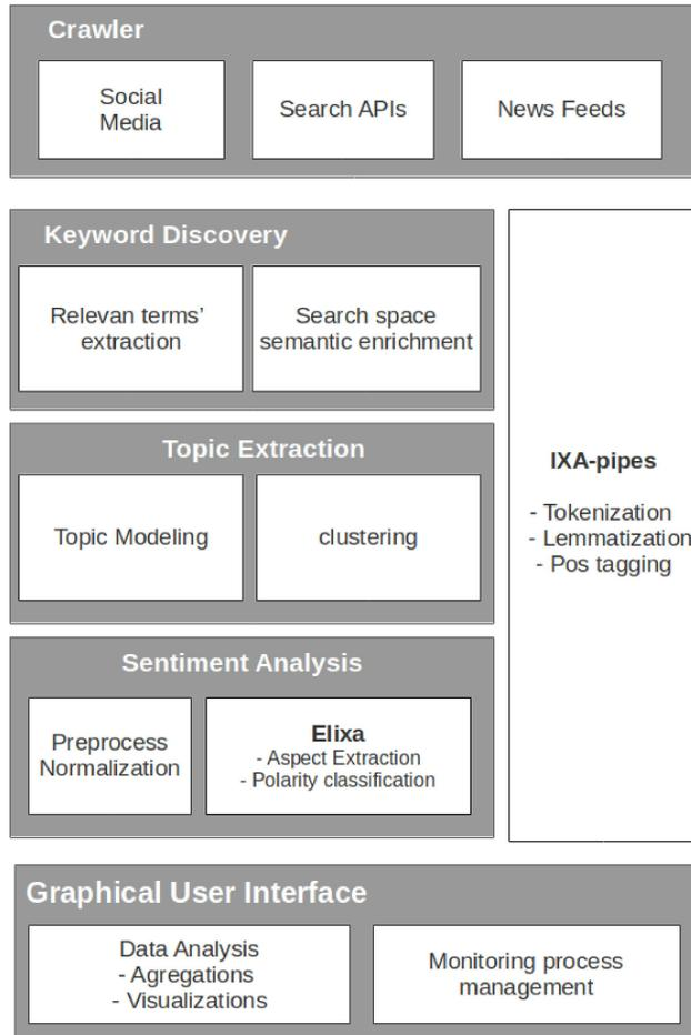
Figure 1: Diagram Talaia's components.
