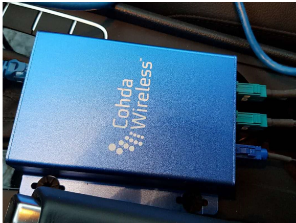
Fig. 2. DSRC radio unit used for our prototype system, manufactured by Cohda Wireless.
