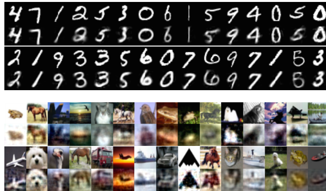
Figure 5.4: Autoencoder reconstructions of unseen test images for the MNIST (top) and CIFAR-10 (bottom) datasets.
