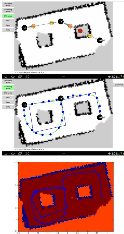
Fig. 9: Experiment 2: LTL specification, sketched path and resulting trajectory. The LTL specification is  $(q_0 \wedge \mathbf{GF}(q_1 \wedge \mathbf{F}q_2))$ .
