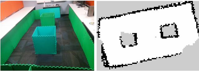
Fig. 7: The experiment environment and its scanned map
