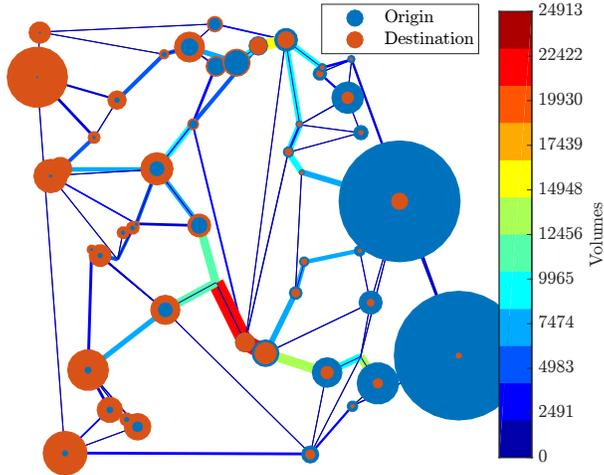
Figure 2: Simulated road networks with the projection of  $\underline{q}$  on the links: the width is proportional to the flows, also correlated with the color. For nodes, the color distinguishes between origin (blue) and destination flows (red) and the diameter of the nodes is proportional to their value in  $\underline{p}_O$  and  $\underline{p}_D$ .
