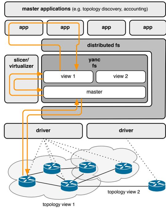
Figure 1: System Architecture
