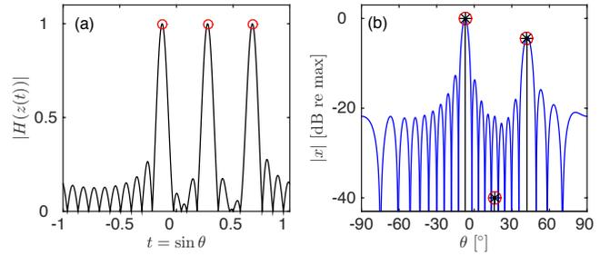
FIG. 3. (Color online) Grid-free sparse reconstruction. A standard ULA is used with  $M = 21$  sensors and  $d/\lambda = 1/2$  to localize three sources (o) at  $\theta = [-7.2385^\circ, 15.962^\circ, 42.0671^\circ]$  with amplitudes  $|x| = [1, 0.01, 0.6]$ . (a) The dual polynomial. (b) Reconstruction with grid-free CS (\*) and CBF.
