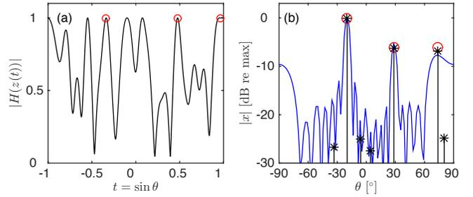
FIG. 6. (Color online) Grid-free sparse reconstruction. A ULA is used with  $M = 21$  sensors and  $d/\lambda = 1/2$  to localize three sources (o) at  $\theta = [-19.6942^\circ, 28.3594^\circ, 73.9457^\circ]$  with amplitudes  $|x| = [0.6, 0.3, 0.3]$ . (a) The dual polynomial. (b) Reconstruction with grid-free CS (\*) and CBF. The SNR is 20 dB.
