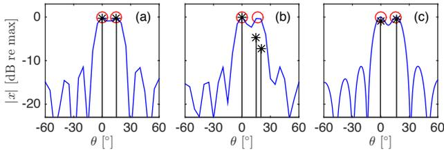
FIG. 1. (Color online) CS performance in DOA estimation in terms of the discretization of the angular space. A standard ULA is used with  $M=8$  sensors,  $d/\lambda = 1/2$  and  $\text{SNR} = 20$  dB. CBF and CS (\*) reconstruction of two sources (o) (a) at  $0^\circ$  and  $15^\circ$  on a grid  $[-90^\circ:5^\circ:90^\circ]$ , (b) at  $0^\circ$  and  $17^\circ$  on a grid  $[-90^\circ:5^\circ:90^\circ]$  and (c) at  $0^\circ$  and  $17^\circ$  on a grid  $[-90^\circ:1^\circ:90^\circ]$ .
