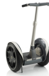
Fig.5. The Segway: A mobile wheeled inverted pendulum [139]
