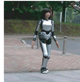
Fig.6. HRP-4C Humanoid: stable walking under linear inverted pendulum model [150]
