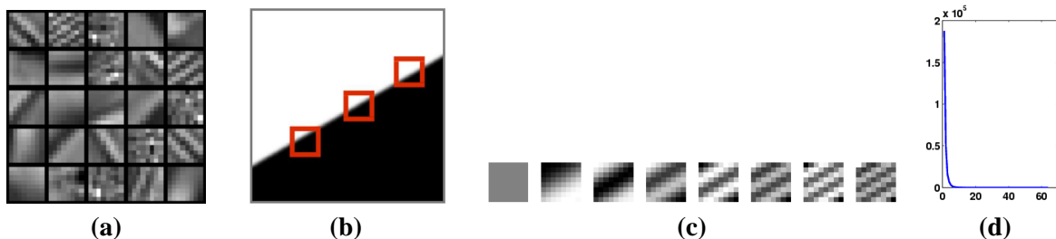
Fig. 2. (a) Some typical dictionary atoms learned from the image Lena (Figure 3-(a)) with K-SVD [2]. (b)-(d) A numerical procedure to obtain the initial directional PCAs. (b) A synthetic edge image. Patches ( 8 \times 8 ) that touch the edge are used to calculate an initial PCA basis. (c) The first 8 atoms in the PCA basis with the largest eigenvalues. (d) Typical eigenvalues.
