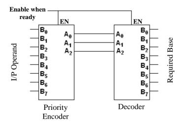
The base calculator allows determination of required base in one clock cycle.
