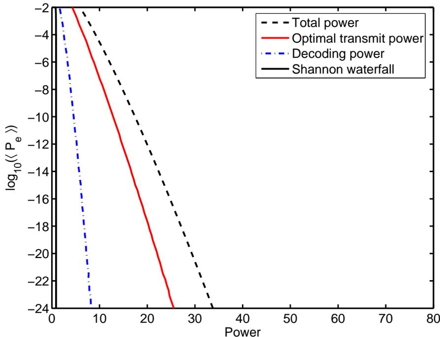
Fig. 3. The waterslide curves for transmit power, decoding power, and the total power for convolutional codes of rate  $R = 1/3$  used with Viterbi decoding. It is assumed that the normalized energy required per operation at the decoder is  $E = 0.3$  and that it takes  $2^{L_c R} \times L_c R$  operations per channel output to decode using Viterbi search for a constraint length of  $L_c$  channel uses.
