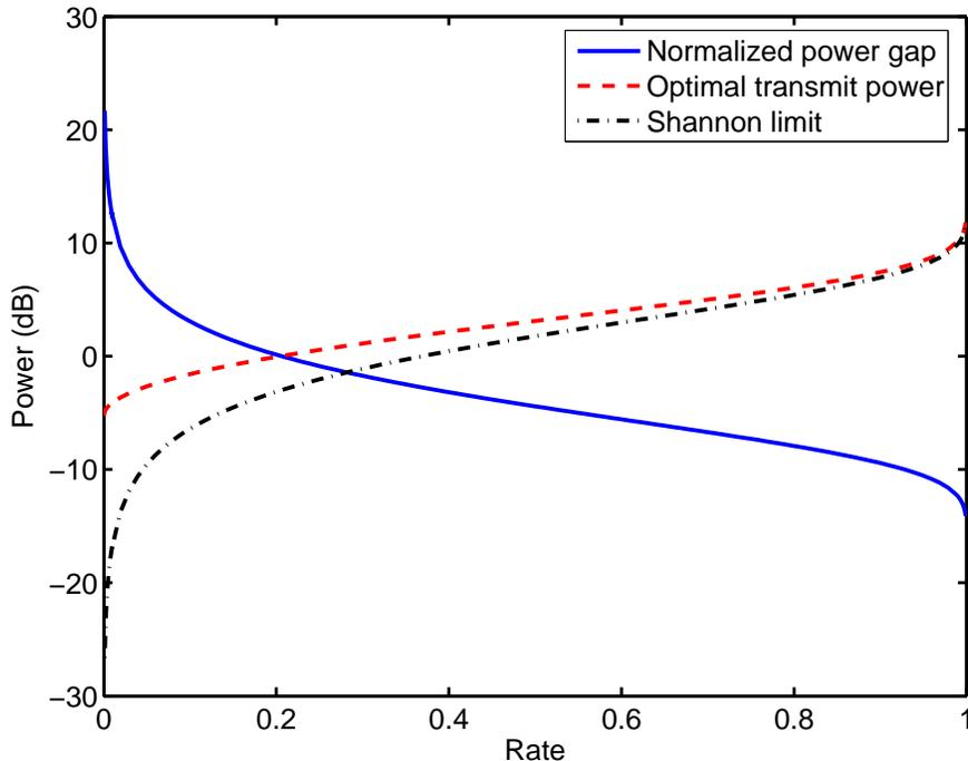
Fig. 10. The impact of rate  $R$  on the heuristically predicted optimum transmit power for  $\gamma = 0.3$ . The plot shows the Shannon minimum power, our predictions, and the ratio of the difference between the two to the Shannon minimum. Notice that the predicted extra power is very substantial at low data rates.
