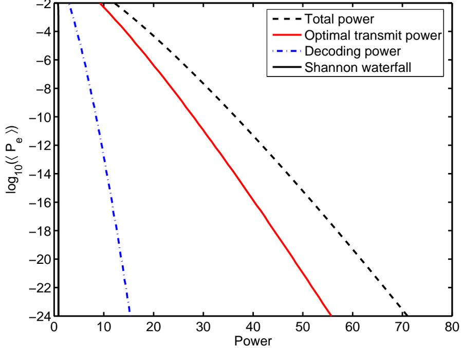
Fig. 2. The waterslide curves for transmit power, decoding power, and the total power for dense linear block-codes of rate  $R = 1/3$  under brute-force ML decoding. It is assumed that the normalized energy required per operation at the decoder is  $E = 0.3$  and that it takes  $2^{mR} \times mR$  operations per channel output to decode using nearest-neighbor search for a block length of  $m$  channel uses.
