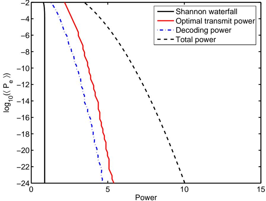
Fig. 4. The waterslide curves for transmit power, decoding power, and the total power for convolutional codes of rate  $R = 1/3$  used with “magical” sequential decoding. It is assumed that the normalized energy required per operation at the decoder is  $E = 0.3$  and that the decoding requires just  $L_c R$  operations per channel output.
