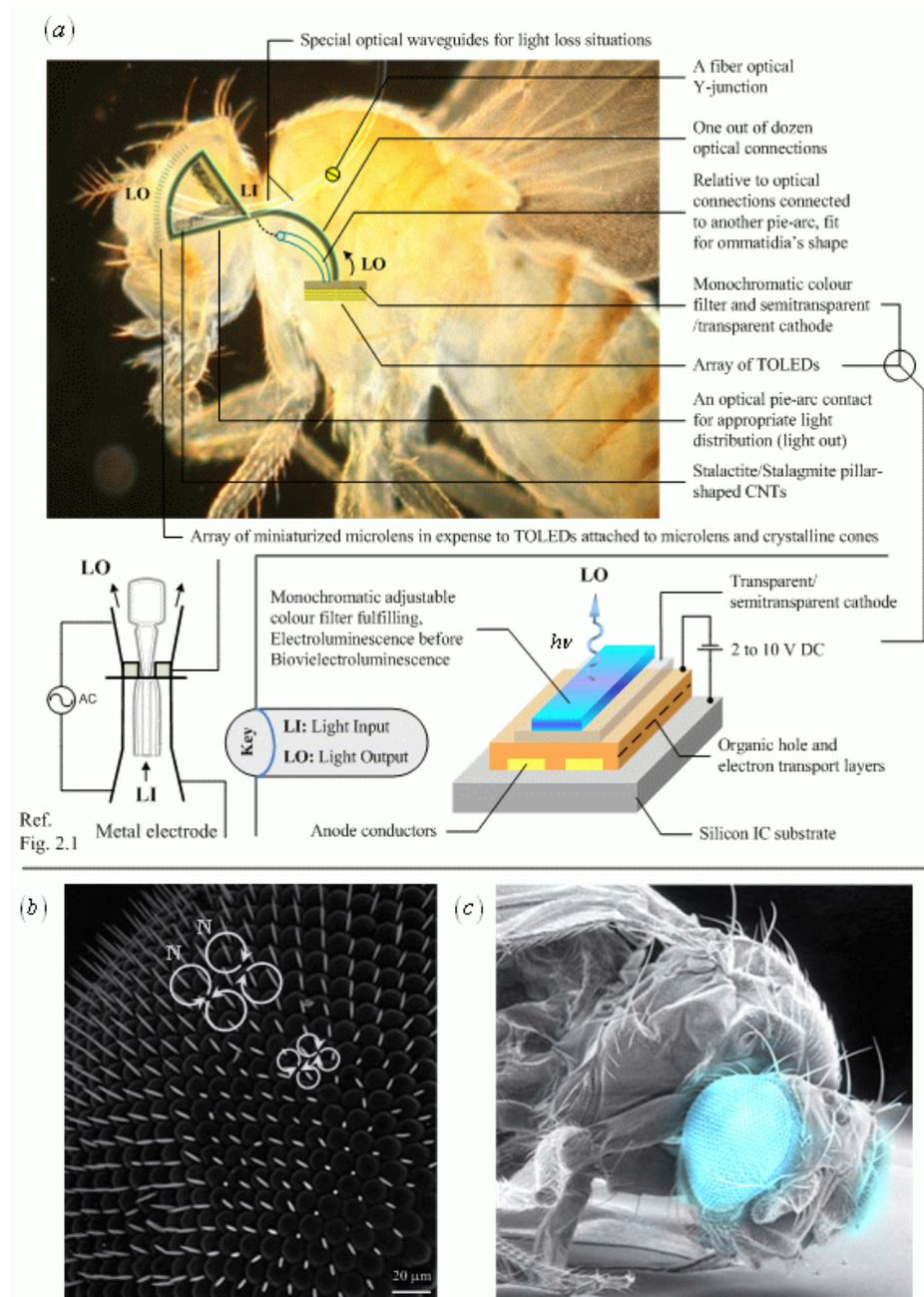
**Figure 2.2.** (a) Cross section installation and insertion technique of optical contacts including, monochromatic top-emitting OLED [54] array, and stalactite/stalagmite angular positioning of pillar-CNTs in the fruit fly's body. The contacts connect from RGB filter to fly's anterior for the diagram illustrated in Fig.2.1. The anatomy of an element of the array as a TOLED with a monochromatic light output is also shown. The given
