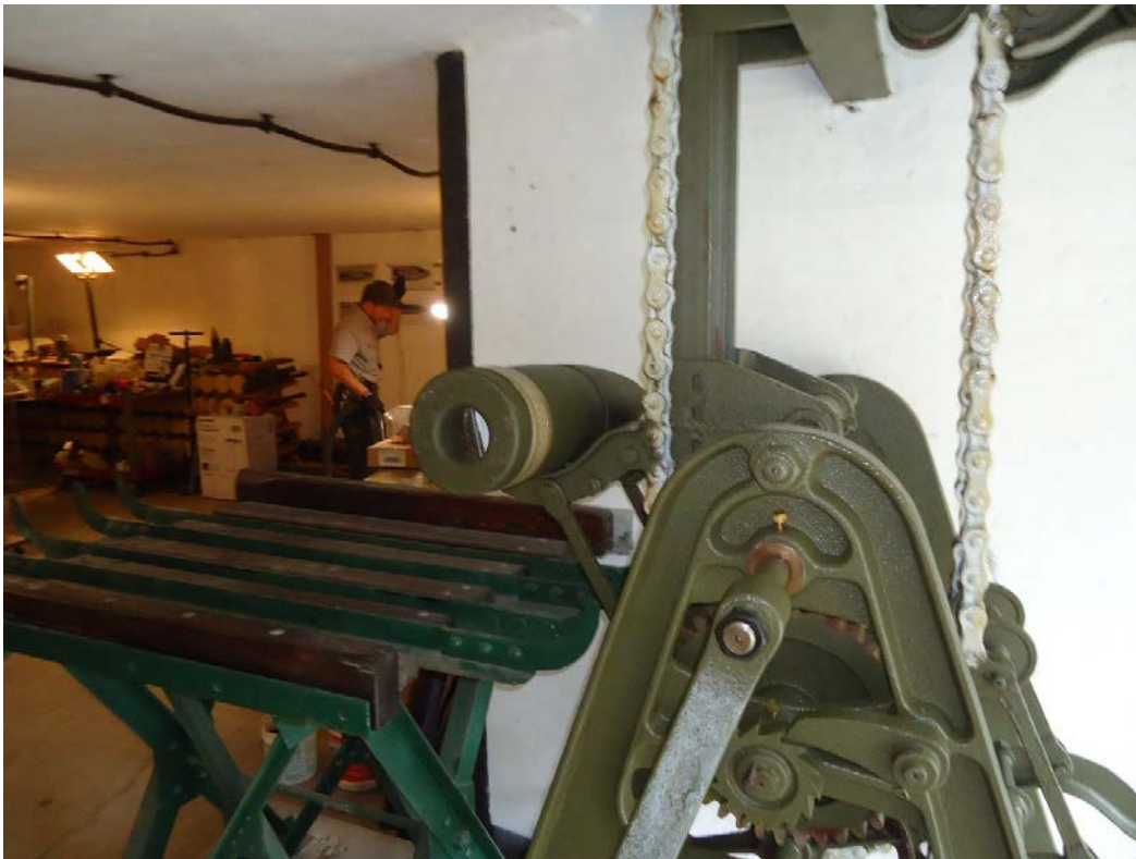
Another view of the drill shell on the hoist lift forks.
