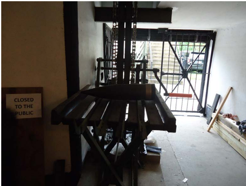
The photo below shows the hoist with the shell table mounted in place.
