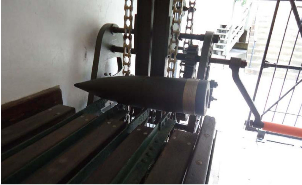
Another view of the drill shell on the hoist lift forks.
