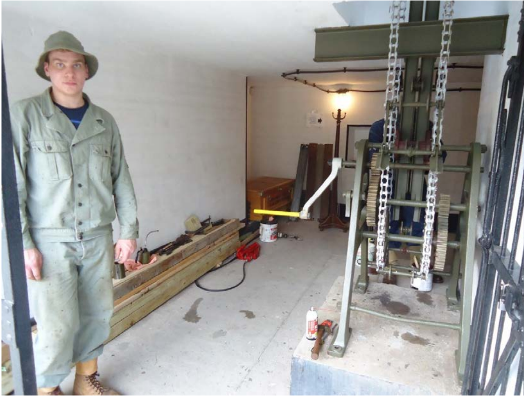
The photo below shows the hoist with the shell table mounted in place.
