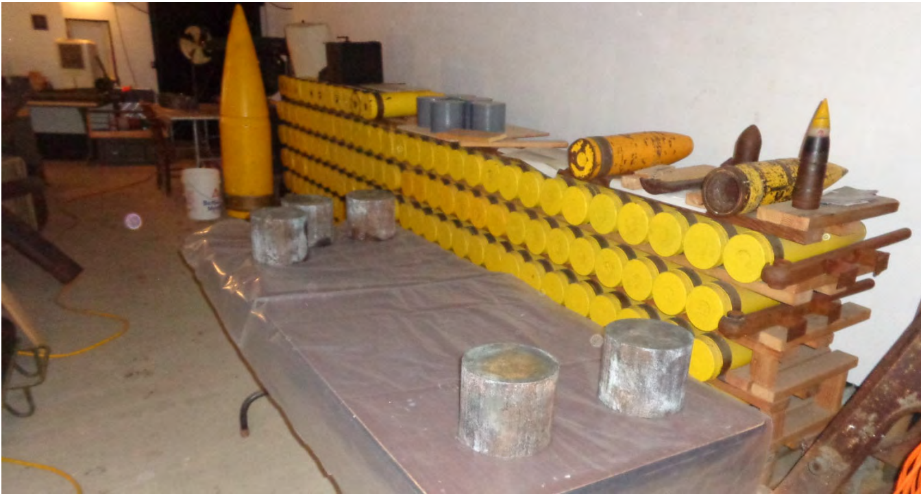
Below are the slugs ready for application of POR-15.
