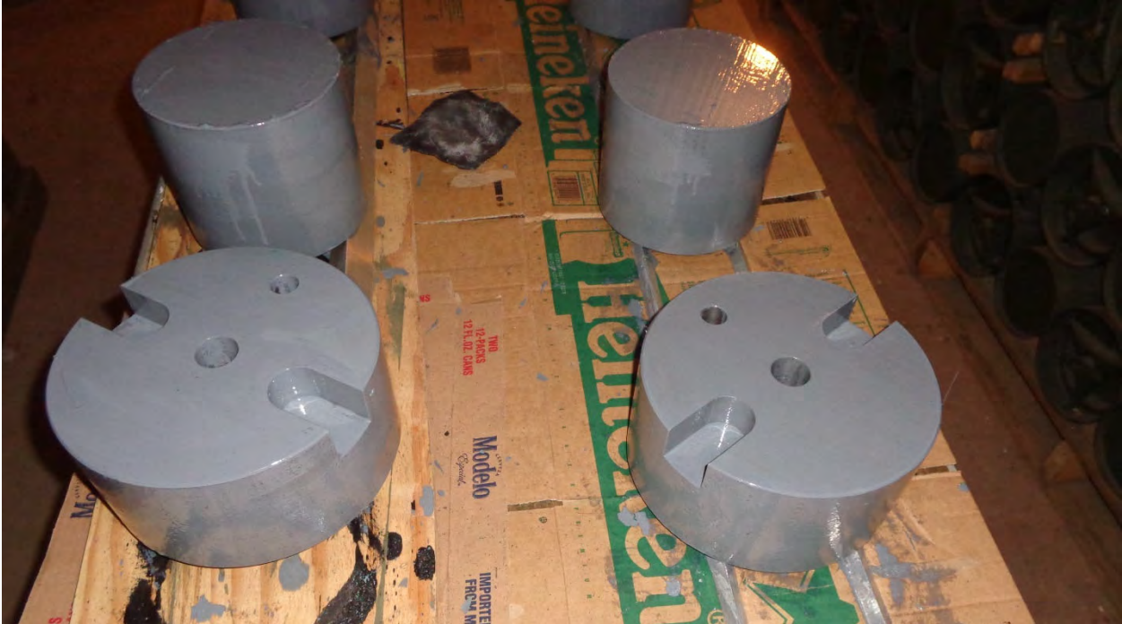
Below is another view of the slugs after treatment with POR-15.
