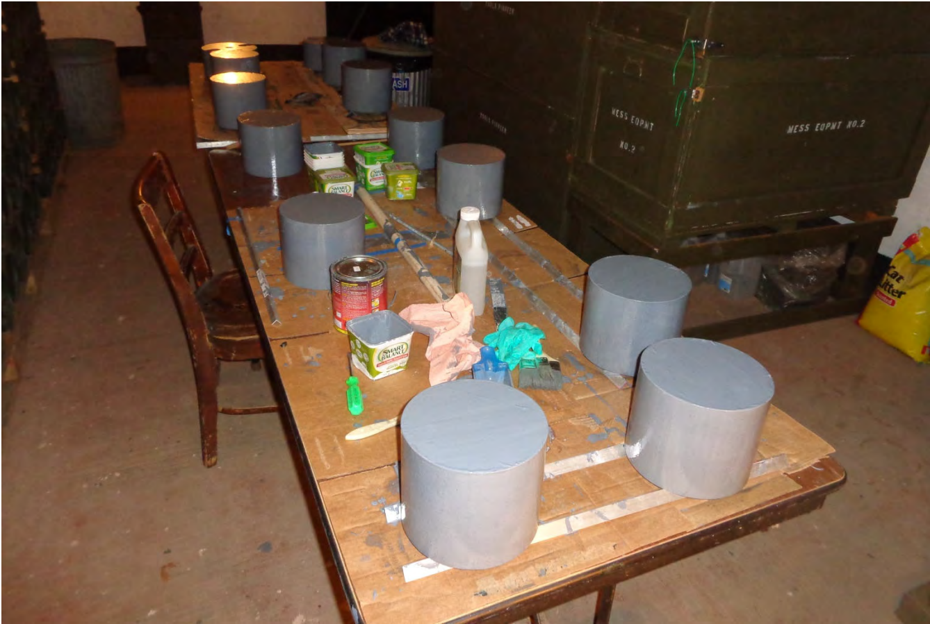
Below is another view of the slugs after treatment with POR-15.
