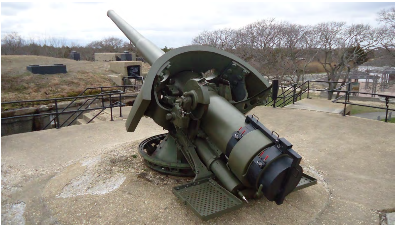
The photo below shows Gun #2 with elevation lock and yoke in place.
