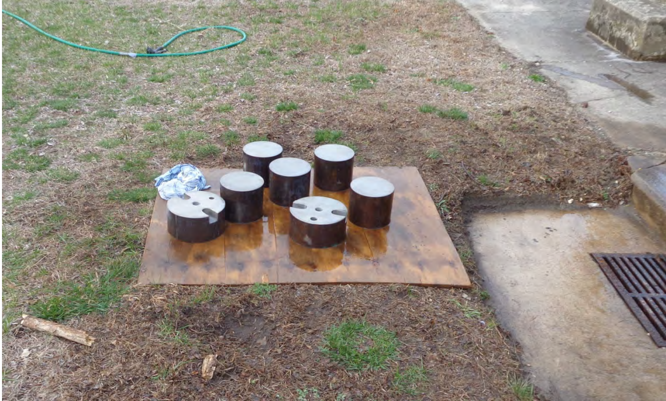
Below are the slugs ready for application of POR-15.
