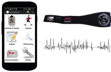
Figure 2. The MobiGuide app; ECG sensor with chest belt, and an atrial fibrillation event detected by the ECG sensor.
