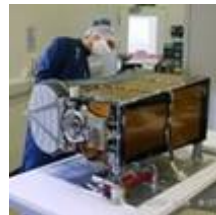
TopSat (Qinetiq-SSTL, GB) 115 kg, 20M$ all included , with amazing operational performances 2.6m resolution 2.6m, 5 yrs life duration expected, agility, direct user...
