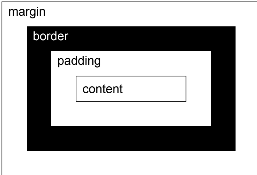
Figure 4: The CSS box model.
