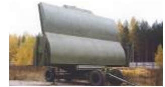
VNIIRT Gamma DE L-band high power AESA search radar in deployed configuration.
