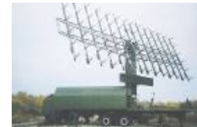
The new 3 dimensional NNIRT 1L119 Nebo SVU AESA is an improved new technology VHF band SAM battery acquisition radars
