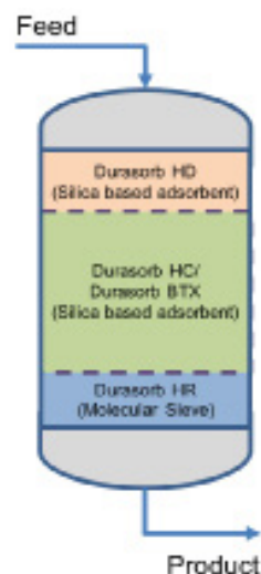
Figure 7. Typical adsorbent bed configuration of BASF Durasorb technology in a dual-purpose concept.
