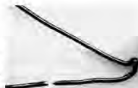
Type S Thermocouple exhibiting grain growth & slippage producing early failure. Surface contamination is evident in one leg near the junction.
