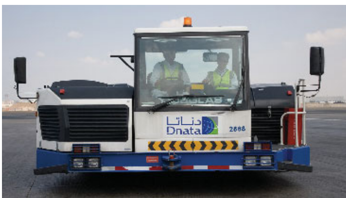
Dnata's new aircraft pushback and towing vehicle, TBL600
