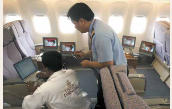
Engineering personnel upgrading the entertainment system on a Boeing 777-200.
