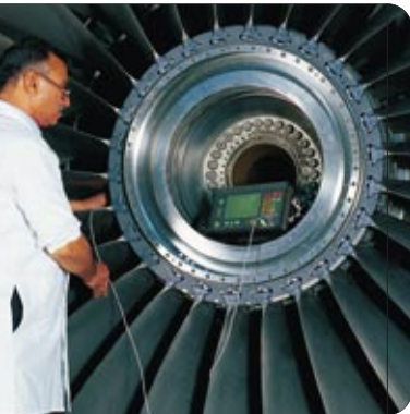
Full module replacement on Rolls Royce Trent 700 and 800 engines.
