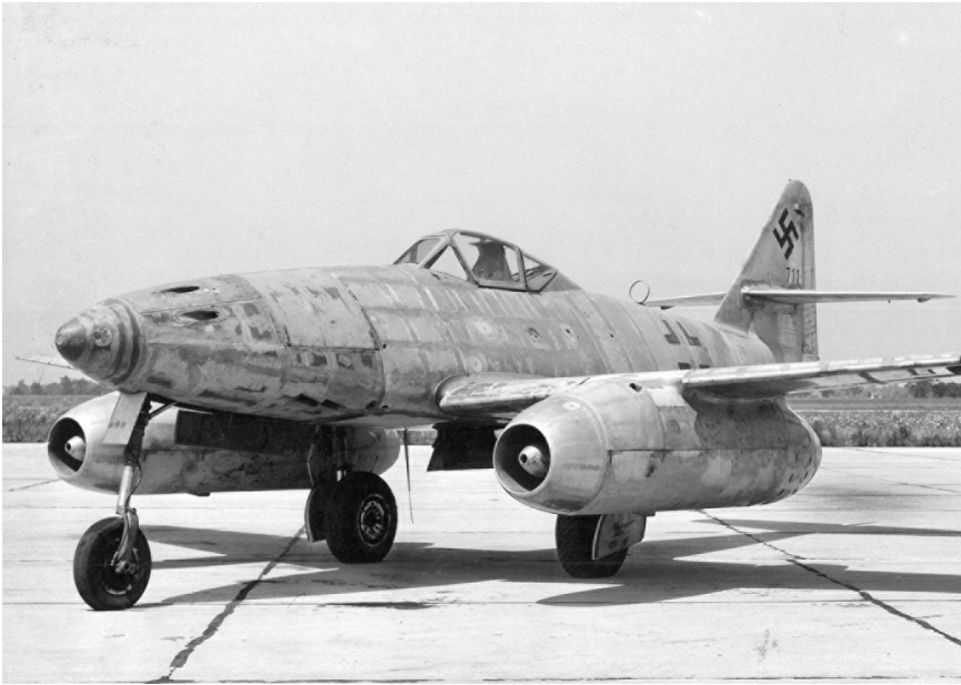
Messerschmitt Me 262 A-1 Jet Fighter. Sightings of the Me 262, which was capable of flying more than 500 miles per hour—over a hundred miles per hour faster than any Allied piston-engine fighter—were of great interest to the provisional air force’s pilots and intelligence staffers. National Archives.
