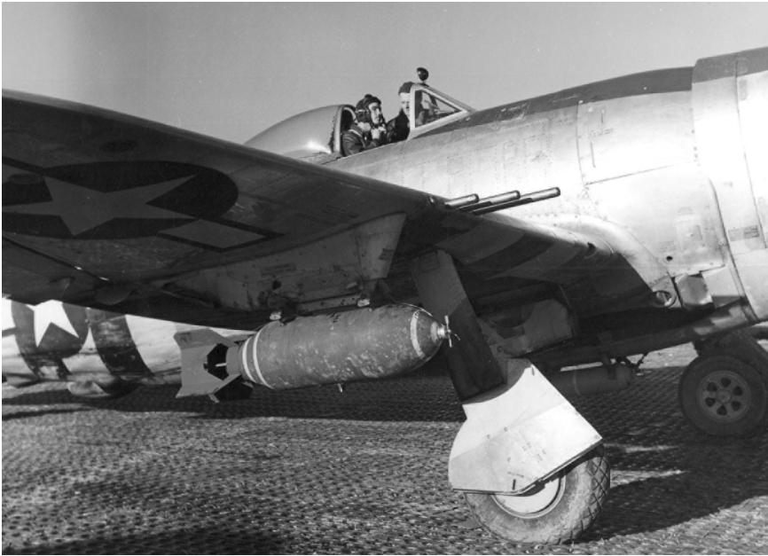
USAAF P-47 Armed and Ready. Crew chief SSgt. John A. Randy prepares pilot Lt. Wilson C. Hansard for a mission. The fighter-bomber's visible external armament includes a 500-pound general purpose bomb underneath the wing and a 100-pound white phosphorus incendiary munition mounted centerline under the fuselage, in addition to its wing-mounted .50-caliber machine guns. National Archives.
