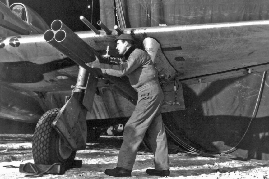
Rocket Launcher-Equipped P-47. Some of the First Tactical Air Force (Provisional)'s fighter-bomber groups received rocket launchers at the end of January 1945, improving their ability to strike trains, vehicles, and troop positions. Here, an armorer works on the launching tubes of one of the 324th Fighter Group's P-47s. National Archives.
