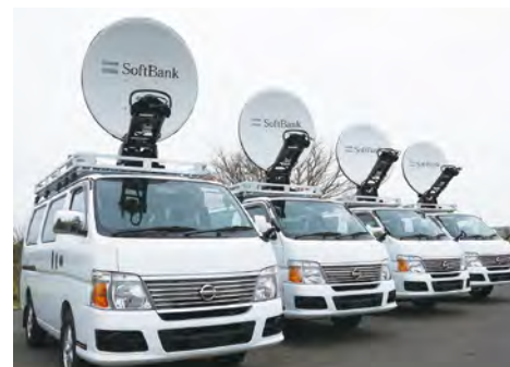
Portable mobile base stations
