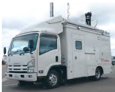
Mobile Base Station Vehicle
