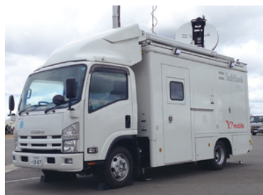
Mobile base station vehicle
