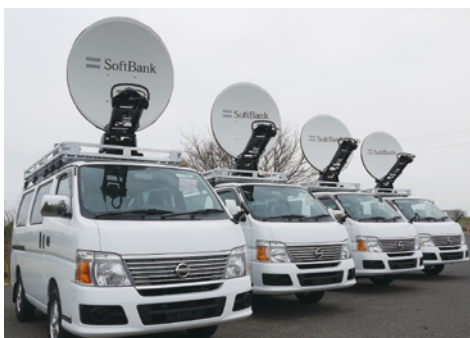
Portable mobile base stations
