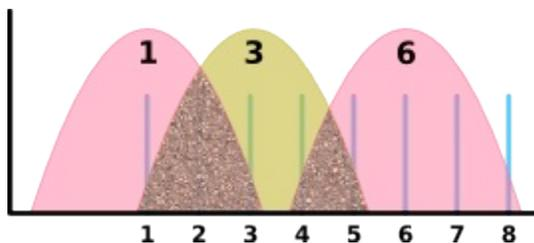
You could use other sets of Wi-Fi channels, as long as they are 5 channels apart - for instance 3, 8 and 13. This may not be optimal though, as channels 1 and 2 would be unused, and in many places in the world channel 13 is not available. Wherever you are, try and check what channels are most in use, and plan your network to use a channel that doesn't overlap.
