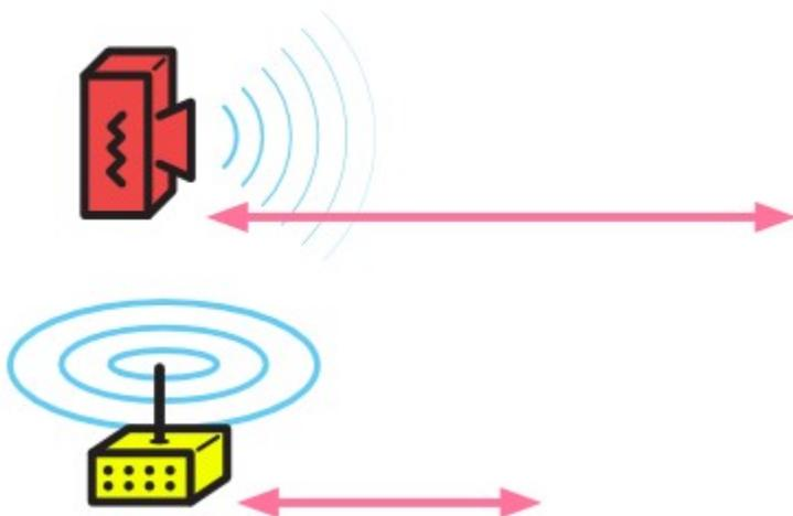
It can also decrease the interference received at the node. There are fewer signals coming in to the antenna, since the node is only listening to signals from the direction it is pointing. It won't hear signals behind it or to the sides as well or at all. This reduces the signals it needs to sort out, and allows it to focus on other signals more, increasing the quality of those connections.
