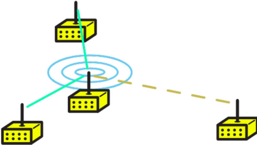
Also, if there are only nodes or clients in one direction of the router, then the signals going in the opposite direction are wasted:
