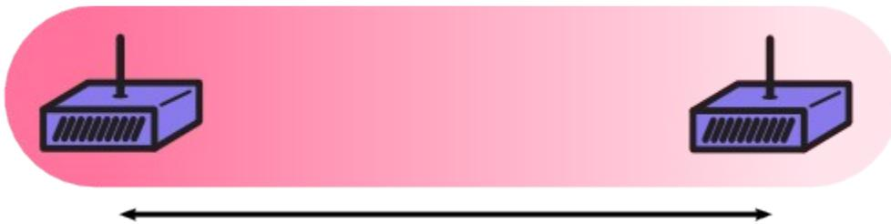
If the router moves too far away from the transmitter, it won't be able to receive any signal, either due to the signal being too weak or other signals interfering, and the routers will disconnect. Below we can see the two routers have disconnected, as there isn't enough signal.
