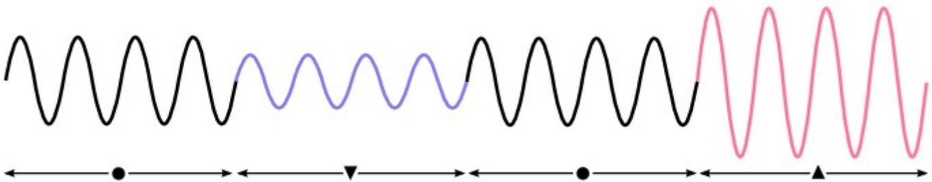
From left to right, we have the normal, un-modulated wave, then the lower amplitude wave (representing low points in audio waves), then the higher amplitude wave (representing crests or high points in audio waves).
