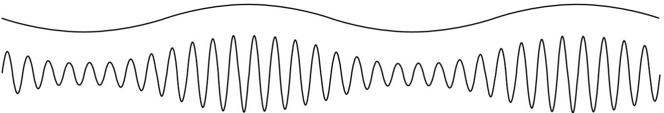
The audio signal is the wave on the top, with the corresponding Amplitude Modulated wave below it.
