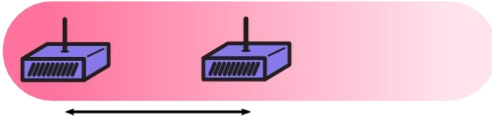
As a receiver moves away from a wireless router, the signal it hears will get “quieter” -- in other words, the power it receives will go down. Below, we can see the same routers, but with more distance between them. In this case, the routers have a weaker connection because the signal is near the limit of what the routers can hear. The speed between the routers will be less.
