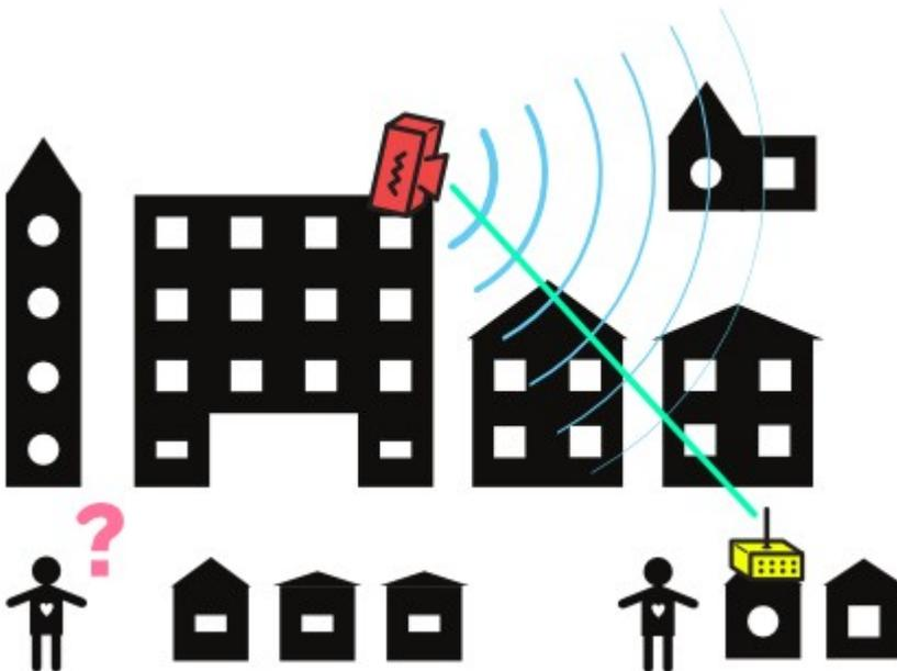
Also, the node has a very powerful signal in a single direction. If omnidirectional units, or lower power units such as laptops, are connecting to the node, they may not connect properly. The laptop will hear the node very well, but the directional node may not hear the laptop. This will create the situation where it looks like there is a strong signal, but you cannot connect.
