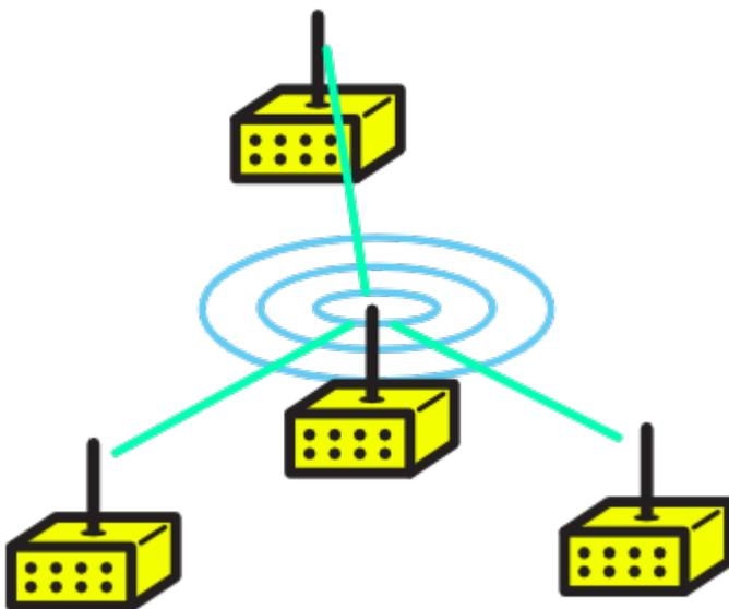
The all-direction strength of these antennas comes with the drawback of transmitting a weaker signal. Since the signal is going in all directions, it spreads out and gets weaker with distance very fast. If nodes or clients are far away, they may not connect well.
