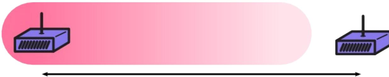
The optimal signal range for outdoor wireless equipment is between -40dBm and -60dBm. This will ensure the connection can maintain the highest bandwidth possible.
