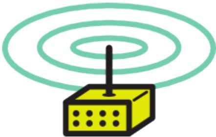
Using omnidirectional antennas has the benefit of creating connections in any direction. You don't have to do as much planning to connect with multiple neighbors or buildings. If there is enough signal between nodes, they should connect.
