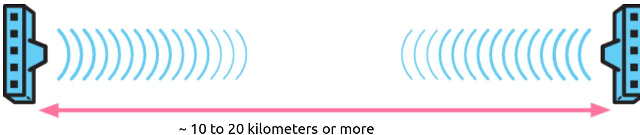
Wireless transmitter power is only one half of the connection. The Wi-Fi receiver has a range of power levels it can hear--the "listen power" in the diagram above. This is also known as the **receive sensitivity**. The receive sensitivity values are generally rated in dBm, and are usually in the range of -40dBm to -80dBm. The negative number indicates a very small signal -- tiny fractions of a milliwatt.
