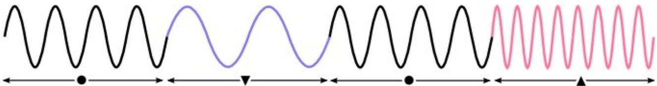
From left to right, we have the normal, un-modulated wave, then the lower frequency wave (representing lower audio amplitudes), then the higher frequency wave (representing higher audio amplitudes).
