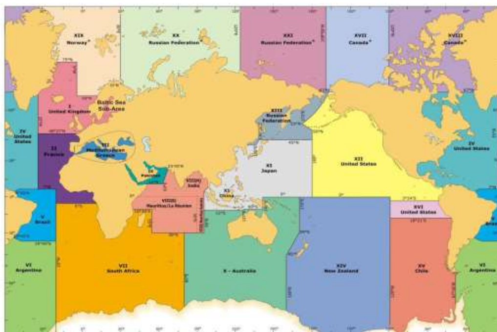
Fig.6.1. AREA OF RESPONSIBILITY AND DESIGNATED NATIONAL METEOROLOGICAL SERVICES FOR THE ISSUE OF WARNINGS AND WEATHER AND SEA BULLETINS FOR THE GMDSS
