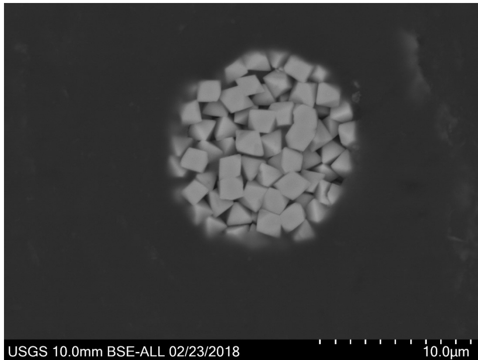
Figure 1.1. Image of a single pyrite framboid. The framboid is composed of an aggregate of approximately 2- \mu\text{m} pyrite crystals that exhibit the octahedral crystal structure of pyrite. The 10- \mu\text{m} -diameter size of the pyrite framboid is typical of Illinois basin coals. Image from sample IL-2, Herrin #6 coal. Abbreviations: BSE-ALL, backscattered electron-image; IL, Illinois; mm, millimeters; \mu\text{m} , micrometers (microns); USGS, U.S. Geological Survey.
