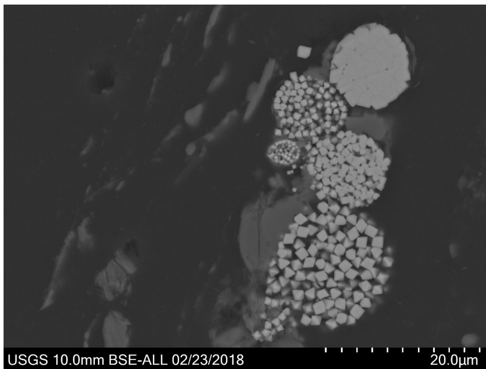
Figure 1.2. Image of a cluster of pyrite framboids from sample IL-2, Herrin #6 coal. Abbreviations: BSE-ALL, backscattered electron-image; IL, Illinois; mm, millimeters; \mu\text{m} , micrometers (microns); USGS, U.S. Geological Survey.
