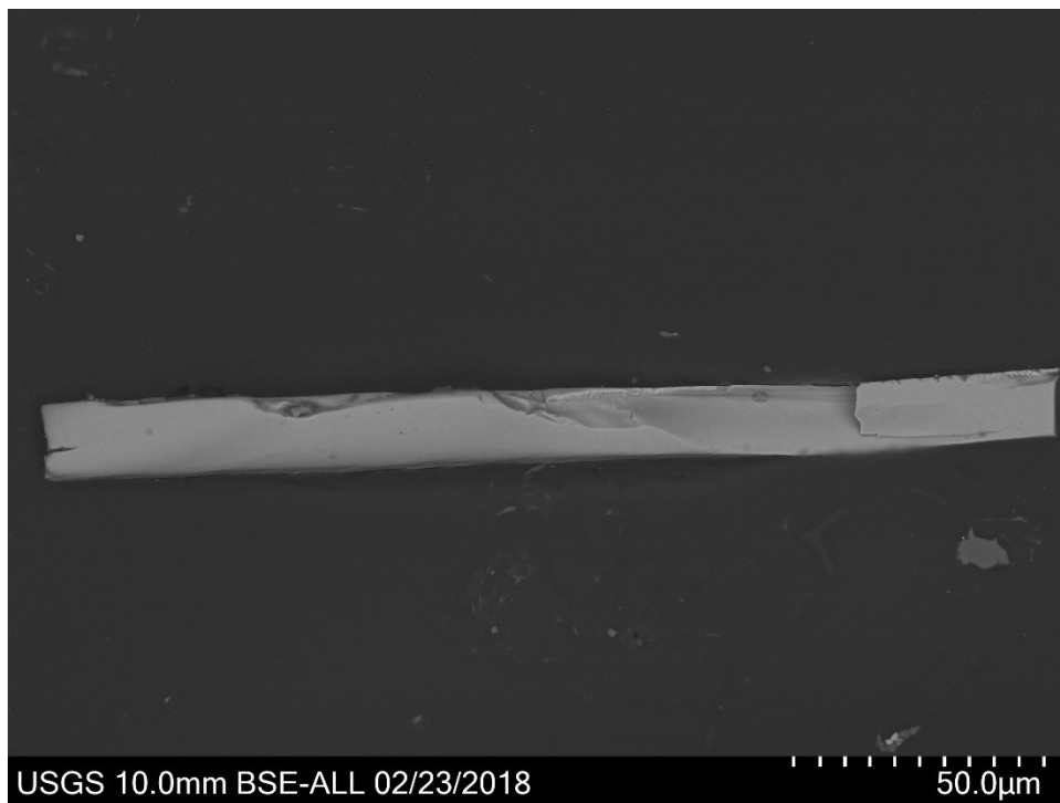
Figure 1.7. Image of a fragment of a secondary pyrite cleat (high contrast) from sample IL-2, Herrin #6 coal. Abbreviations: BSE-ALL, backscattered electron-image; IL, Illinois; mm, millimeters; \mu\text{m} , micrometers (microns); USGS, U.S. Geological Survey.
