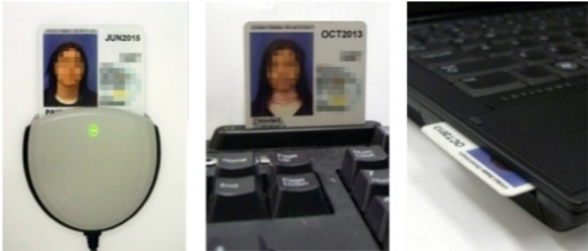
Figure 2: From left to right, a USB smartcard reader, a keyboard reader, and a laptop reader
