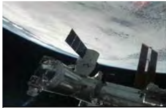
The International Space Station's Canadarm2 installs SpaceX Dragon cargo craft to the Earth facing side of the Harmony node (Credit: NASA)
