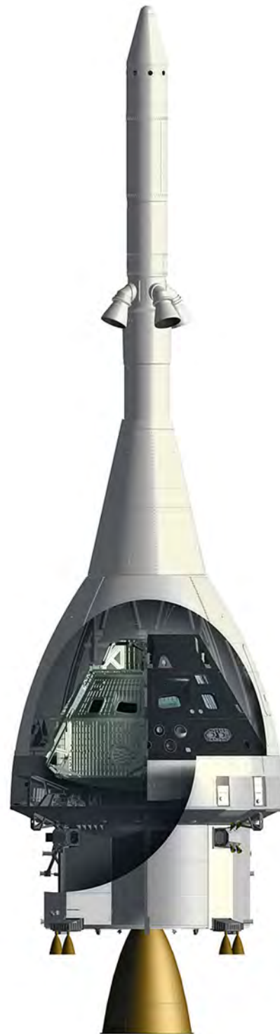
A cutaway of the Orion Multi-Purpose Crew Vehicle (MPCV). The crew module is shrouded inside the Launch Abort System atop the service module. (Credit: NASA)
