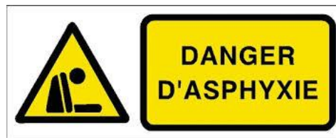
Fig. n° 2: Danger labelling used by gases professionals.
