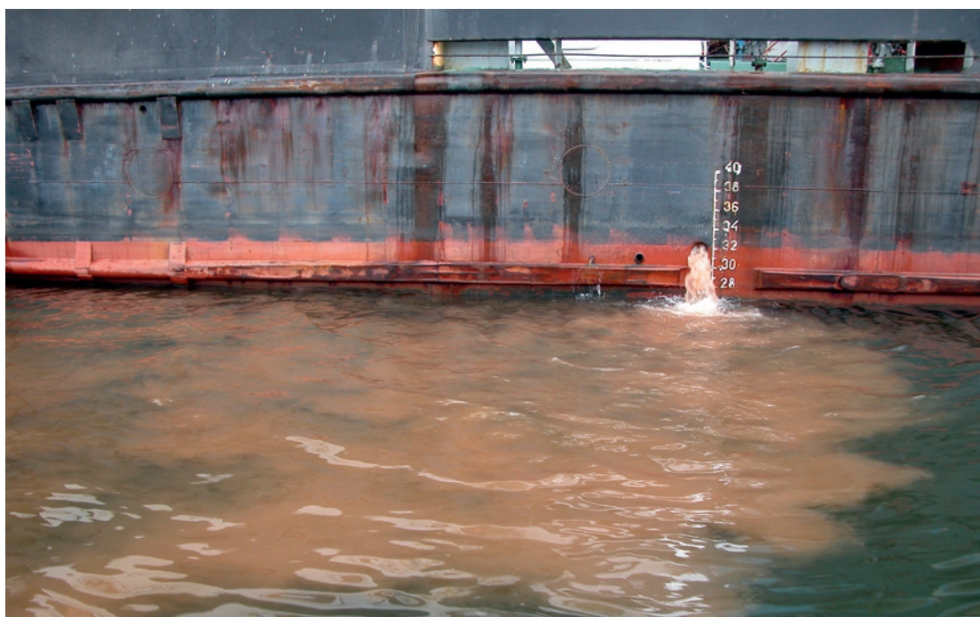
Ballast water has been identified as the vector for spreading many non-indigenous species. Photo: Maritime Office Gdynia.
