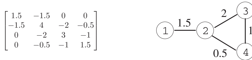
FIG. 1. A Laplacian matrix and its corresponding weighted graph.
