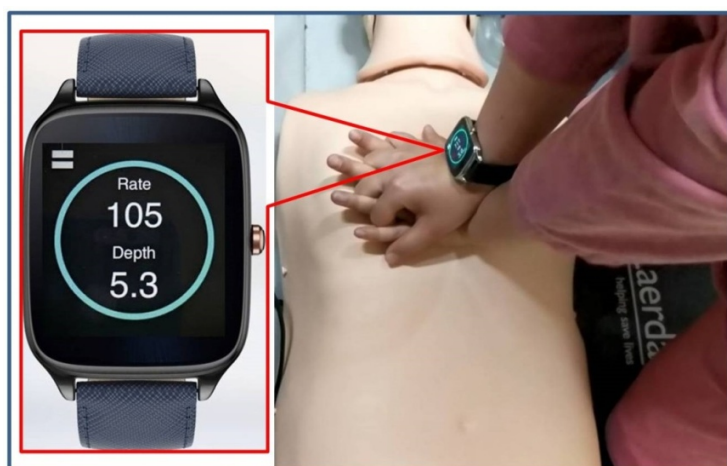
Figure 6.3. Fig. 3. A participant allocated to the intervention group wearing a smartwatch (ASUS ZenWatch 2) with pre-installed app performed chest compression on the manikin.
