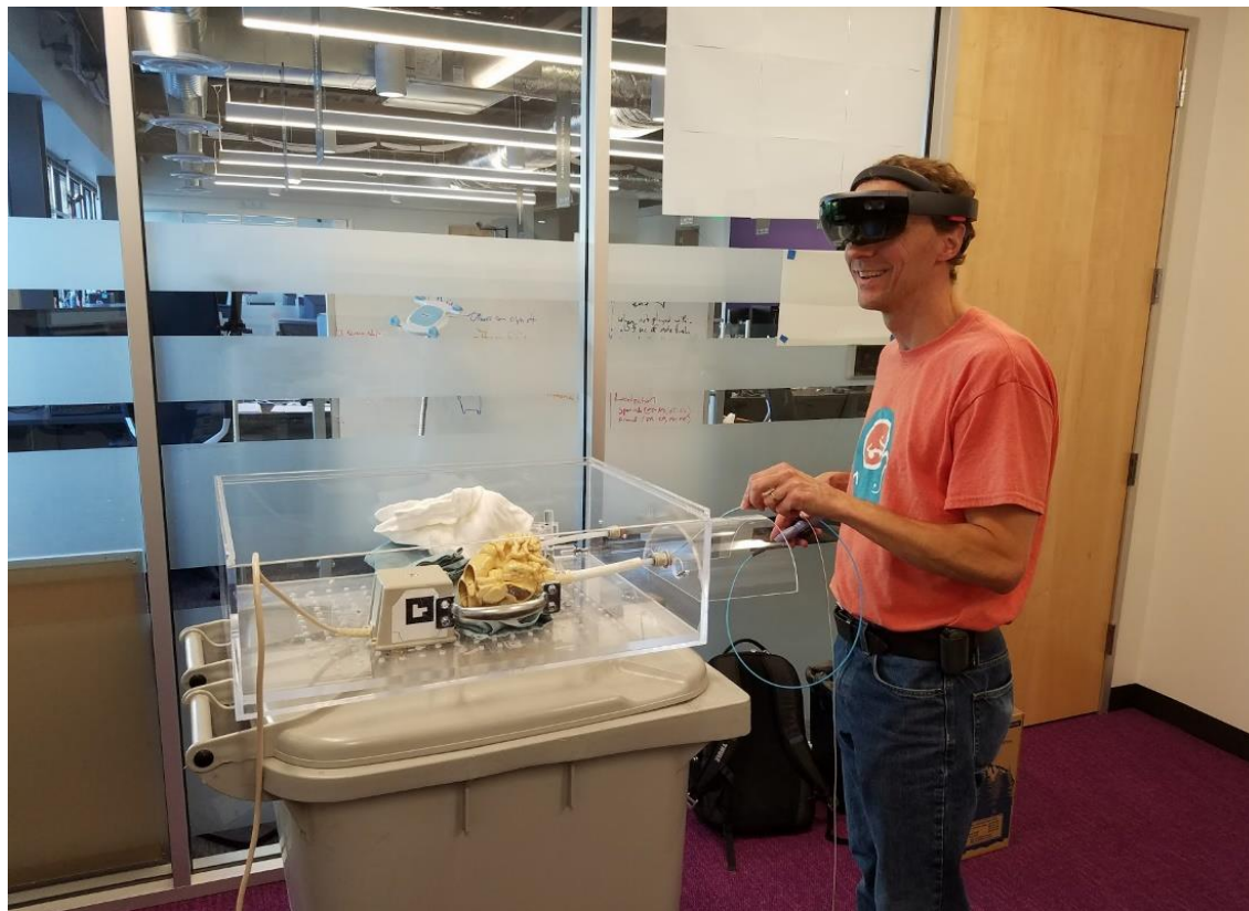
Figure 4.10 Actual image of the first version of CathEye where Dr. Seslar can see holographic navigational information through the HoloLens OSTAR HMD
