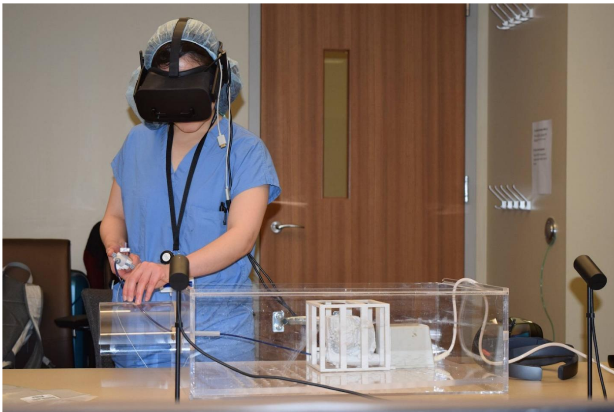
Figure 4.12 An EP at Seattle Children's navigating a catheter while she's surrounded by a virtual rendering of the heart in a VR HMD.
