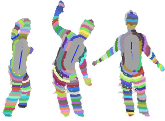
Figure 5: Three examples of narrow band filtering. The obtained regions are randomly painted. In this case, an A^{max} = 70 \text{ cm}^2 has been applied together with a (\eta_L = 30, \delta_L = 4 \text{ cm}) -connectivity.
