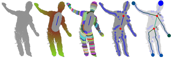
Figure 1: Summary of the steps involved in the proposed algorithm for human pose estimation. From left to right: Foreground mask, R-NBLS propagation, R-NBLS filtering, end-effector graph nodes and end-effectors found with the associated skeleton.
