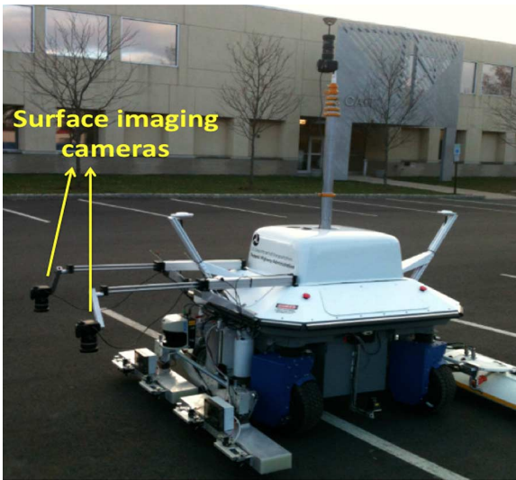
Fig. 5. Seekur robot mounted with cameras used for image collection. The robot is remotely operated and data is sent to the base station located in a van at the end of the bridge-testing area.
