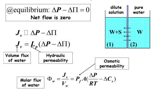
Simulation of osmotic pressure induced water transport may be done by adding salt to one side of the membrane.
