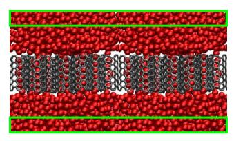
Applying force only on a slab of water in bulk.
