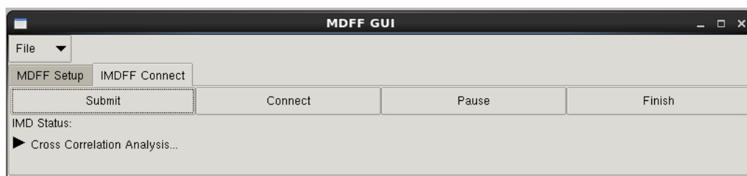
Figure 19: IMDFF Connect tab of the MDFF GUI, where interactive MDFF simulations can be submitted, connected to, paused, terminated, and analyzed
