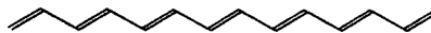
FIG. 1. Ground state of polyenes and polyacetylene characterized by alternating single and double bonds.
